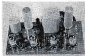
Printed wiring program amplifier.
