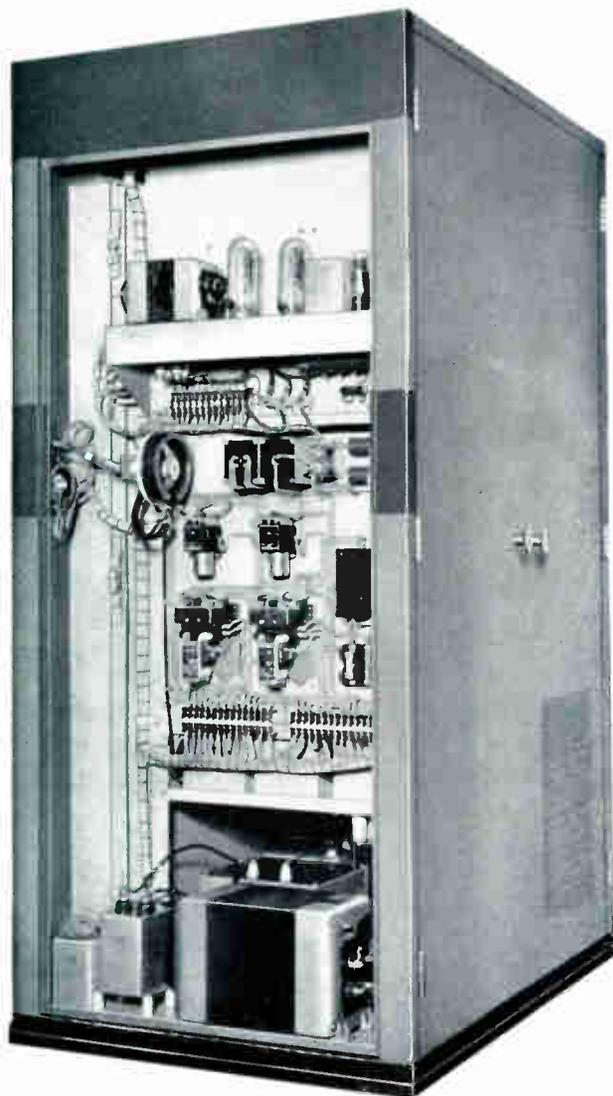
The audio amplifier deck at the top, control panel below and modulation transformer and reactor on the bottom are shown here. Notice the neat arrangement of the components and wiring—not crowded, easy to find your way around. Each electrical part here as well as in other sections of the transmitter is coded to correspond with symbols on the schematic diagram and parts lists in the instruction book.
