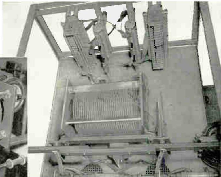
The nitrogen filled tuning capacitors for the final amplifier provide more compact construction than is usually found in apparatus of this type. Due to the fact that they are completely sealed, no insects, dust or other foreign material can enter.
