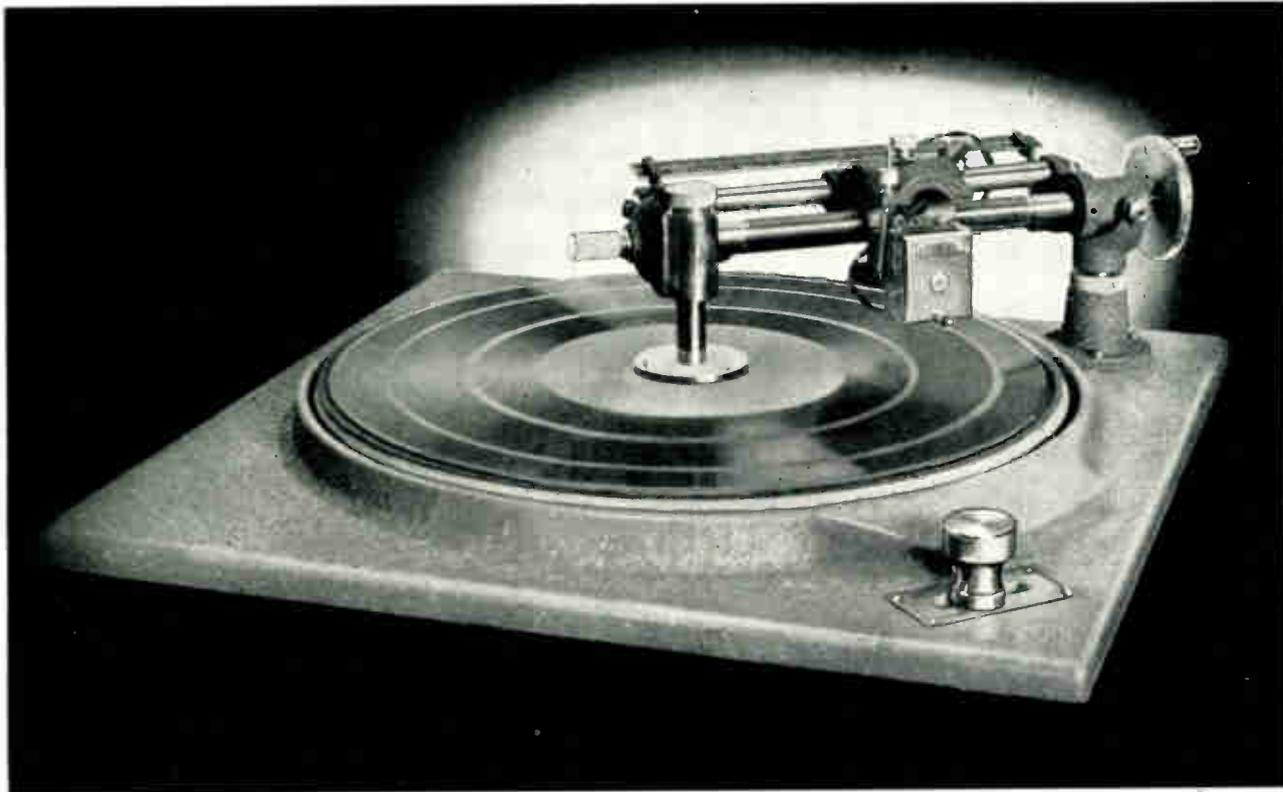
The CB-8R recorder consists of a turntable, overhead feed screw mechanism, cutter head, playback reproducer, microscope and automatic equalizer all mounted into an attractive two tone cabinet of proper height to operate the equipment from a standing position. Either 33 or 78 RPM recordings can be made.
