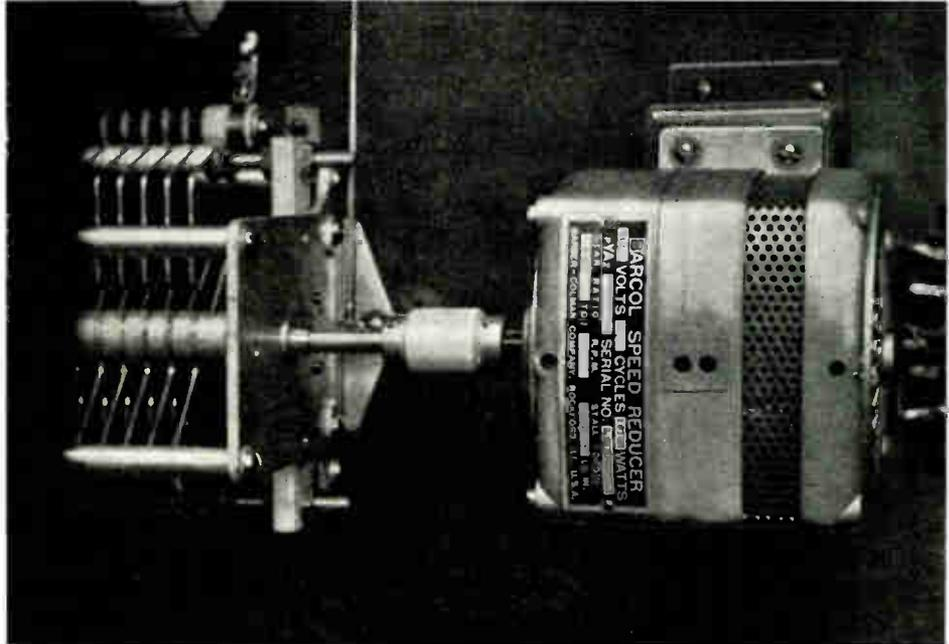
A slow speed motor accomplishes tuning adjustments easily and quickly on the 250C-1 transmitter. Its operation is controlled from the front panel.
