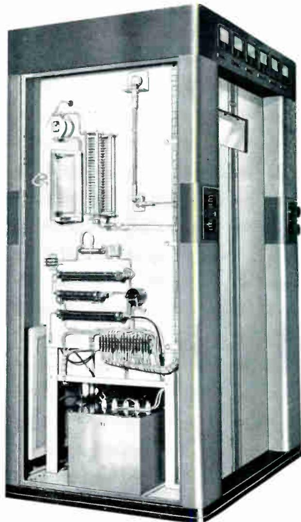
This view shows the output coupling section, large resistors and main power transformer. Notice the intake air filters at the lower left. If desired coaxial line may be brought up through the bottom of the cabinet for convenient termination to the R. F. output.
