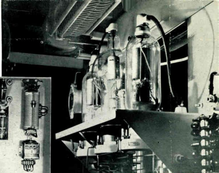
The final amplifier and modulators are shown in the illustration above. A single type 450TH or 250TH may be used for the final amplifier without making any mechanical or electrical changes. The modulators are 810 tubes.
