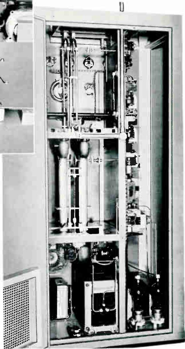
The back of the BF-3A is fully exposed when the rear door is opened. At the top is the  $\frac{3}{4}$  wave length grid tank. Power tubes are located on the top shelf and set into the vertical pipes directly below, which are the final tank circuit. The two blowers exhaust air into these pipes to cool the tubes.
