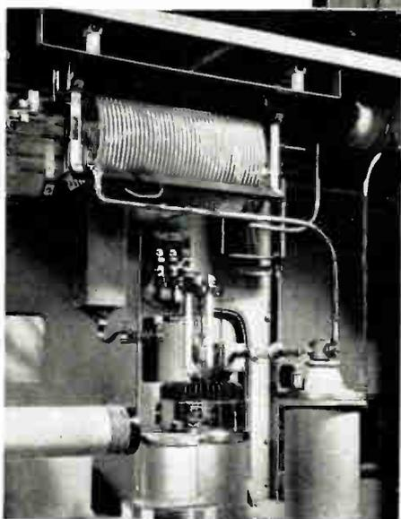
▲ The R.F. amplifier unit, above, is arranged for 5 k.w. operation as it has just a single tube in the final stage. For 10 k.w. operation another socket is installed behind the plate choke and an additional blower, filament, transformer and other minor parts are supplied. The changes are easily and quickly made in the field if necessary.
