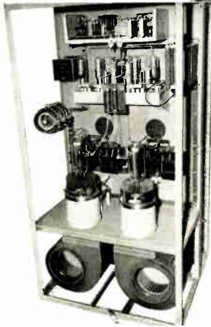
The modulator typifies the open manner of construction used throughout the HF-8 transmitter. Every part is easy to examine and maintain.
