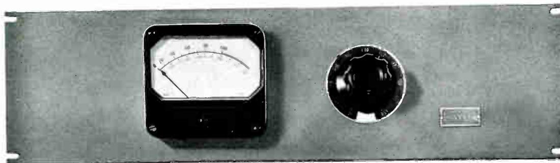
The volume indicator is a necessary part of every radio broadcasting station as well as telephone communications transmitting plant. The main value is reading volume level of the transmitted program but likewise it is equally valuable in taking frequency response measurements, checking level of incoming remote lines and making comparative level measurements of various circuits where the level must be the same.
