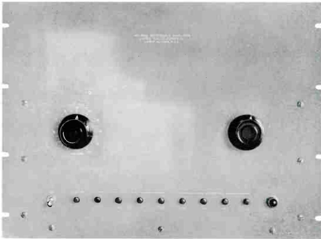
The Model RA-10 Amplifier is designed to produce frequency response curves for making recordings having orthacoustic, standard lateral or straight line fidelity characteristics. A three position switch on the front panel makes any one of the three characteristics available by selecting the proper filter circuit within the amplifier.
