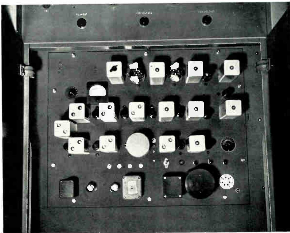
The exciter section shown above, located in the 250 watt cabinet, is the heart of all Gates FM transmitters. In the second row of components, inside the round shield is the 6L-2424 tube which performs the modulation. The modulation inductance is built inside the shield and comes off with it to facilitate tube replacements. The blank socket in the lower right corner accommodates a spare crystal and holder identical to the regular one shown in place adjacent to it.
