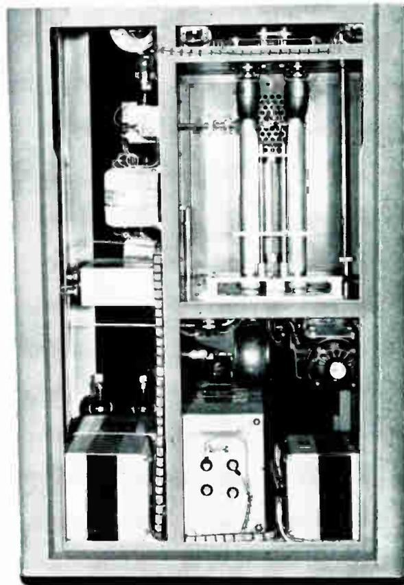
This is approximately the bottom half of the three kilowatt cabinet showing the large power components, blowers and plate tank components.
