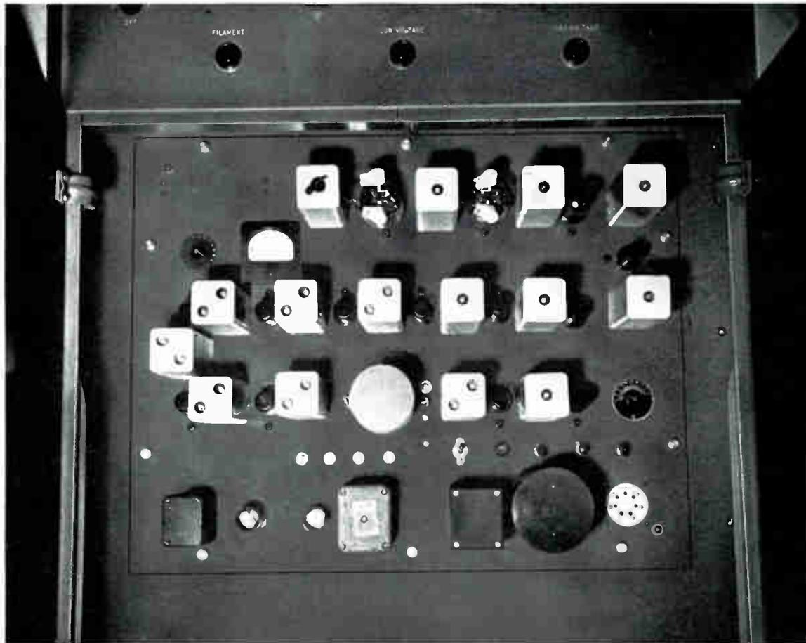
The modulator-amplifier section shown above is the heart of the BF-250A transmitter. In the second row of components inside the round shield is the 6L-2H21 tube which performs the modulation. The modulation inductance is built inside the shield and is easily removable for tube replacements. The blank socket in the lower right corner accommodates the second crystal and oven.
