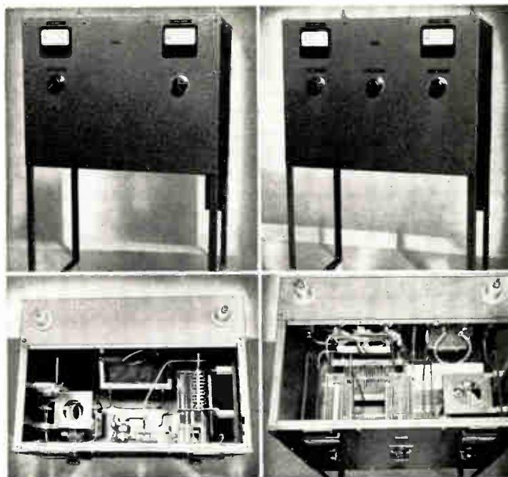
These are front and inside views of the two antenna couplers used with the phaser on the left.
