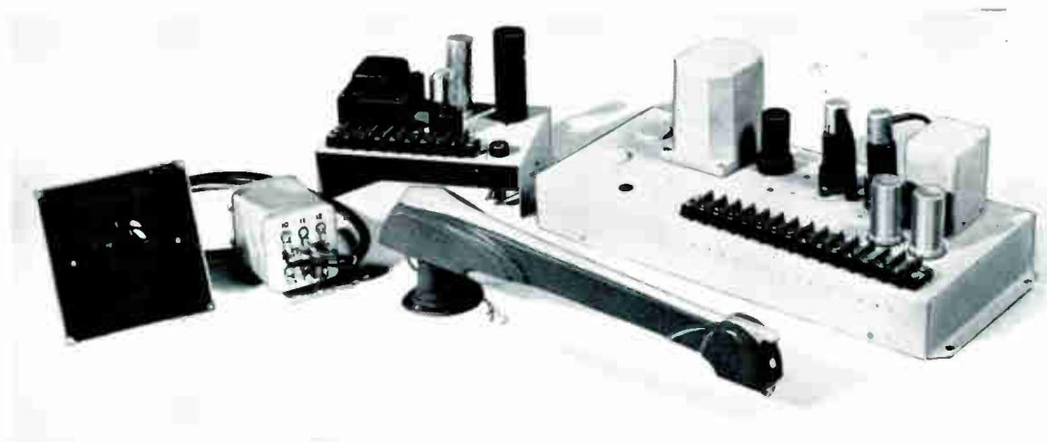
RMC pickup complete with filters, power supply and three stage preamplifier — Selection seven.
