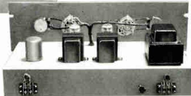
sary for changing alternating current to direct current for application to the plates of the tubes and for biasing purposes. Two large transformers, used to step up the alternating voltage, operate in conjunction with the rectifier and are located adjacent to it.
