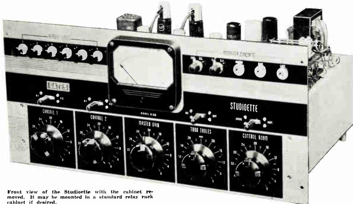
Front view of the Studioette with the cabinet removed. It may be mounted in a standard relay rack cabinet if desired.
