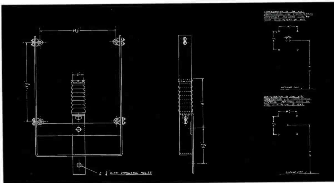
MO-2856 open wire transmission line bracket consists of a steel support formed into the shape of a "U" with a ceramic insulator mounted in the center. All metal surfaces are hot dip galvanized to prevent oxidation. The insulator is designed to accommodate either one or two wires as the current carrying conductors while four clevises are mounted on the
