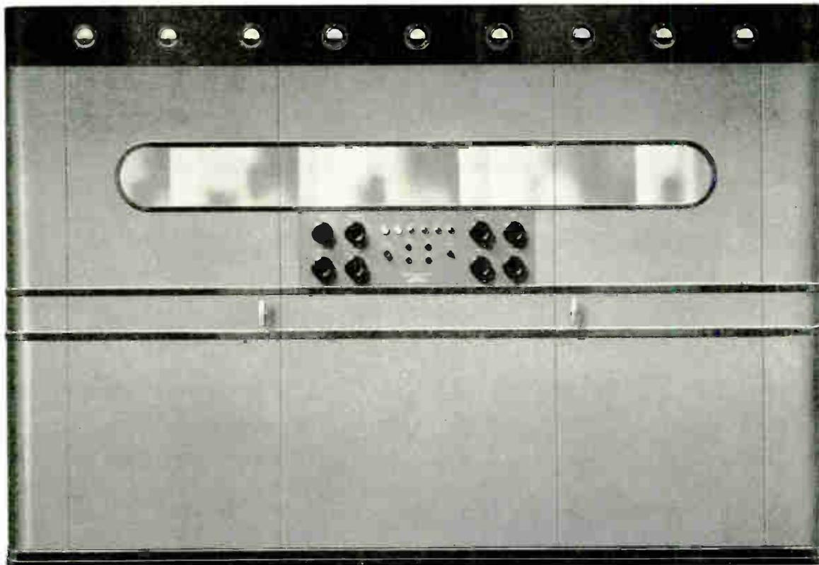
The HF-8 Transmitter is offered to the international communications field to fill high fidelity broadcasting requirements or general communication applications where both radio telephone and high speed radiotelegraph circuits are employed. It has eight kilowatts power output over its frequency range of two to twenty megacycles.
