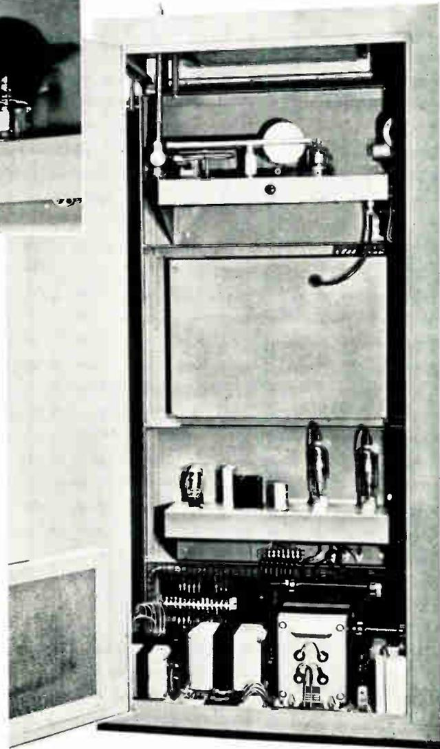
Above is the rear view of the 250 watt exciter. This cabinet and the one on the opposite page ordinarily get side by side to form the complete BF-3A three kilowatt FM transmitter.
