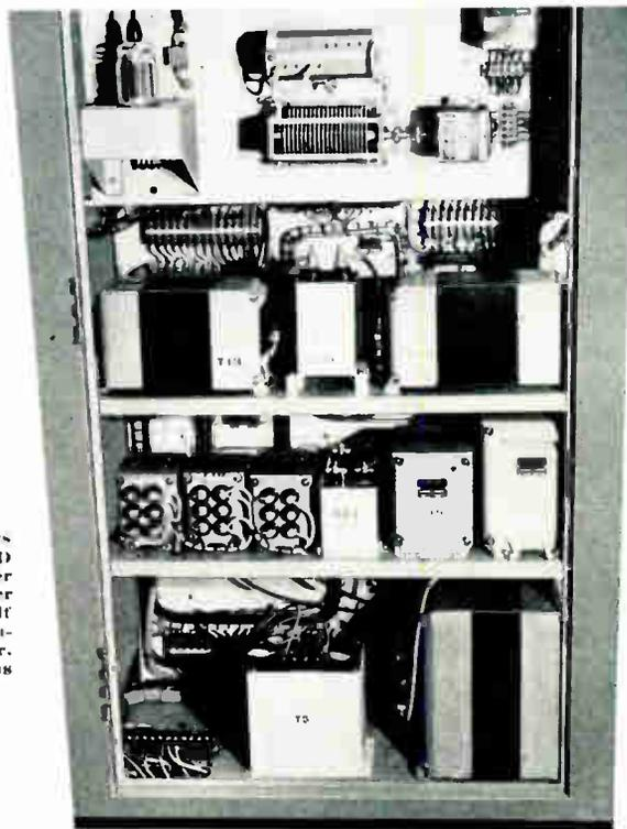
The rear view to the right shows the lower half of the BC-250D transmitter. The main power transformer is in the lower right corner. On the third shelf from the bottom are the modulation transformer and reactor. All are of generous proportions to insure long life.
