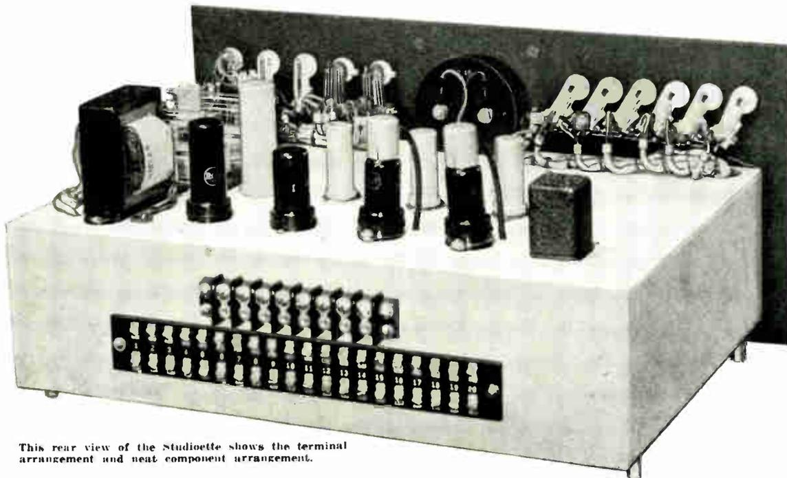
This rear view of the Studioette shows the terminal arrangement and neat component arrangement.
