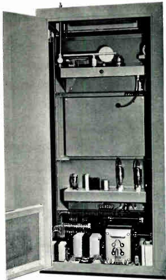
This is the rear view of the 250 watt portion of the BF-1A. The dust cover of the exciter unit in the center of the illustration can be easily removed for exposure of all components. Excitation is carried from the power stage of this cabinet to the grid circuit in the 1000 watt cabinet by a short section of coaxial cable.
