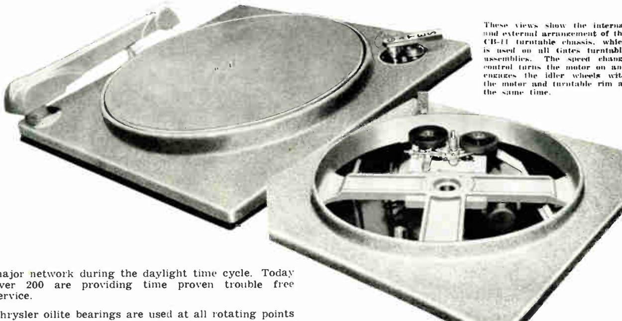
These views show the internal and external arrangement of the CB-11 turntable chassis, which is used on all Gates turntable assemblies. The speed change control turns the motor on and engages the idler wheels with the motor and turntable rim at the same time.
