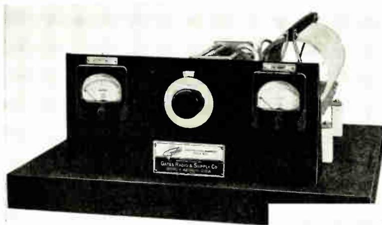
This view of the 21 Series Antenna tuning units shows the front with the cover removed.
