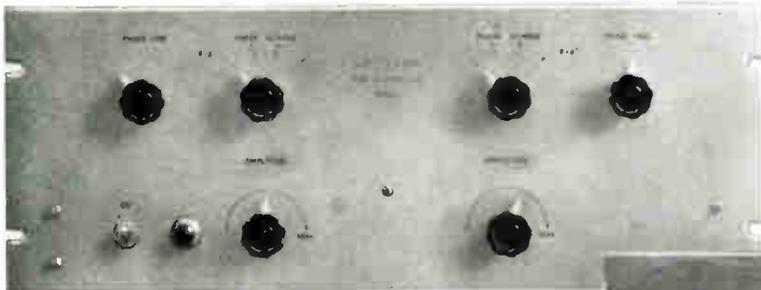
Controls are clearly marked to enable easy adjustment and thus obtain the best results in the Hum Eliminator Amplifier.
