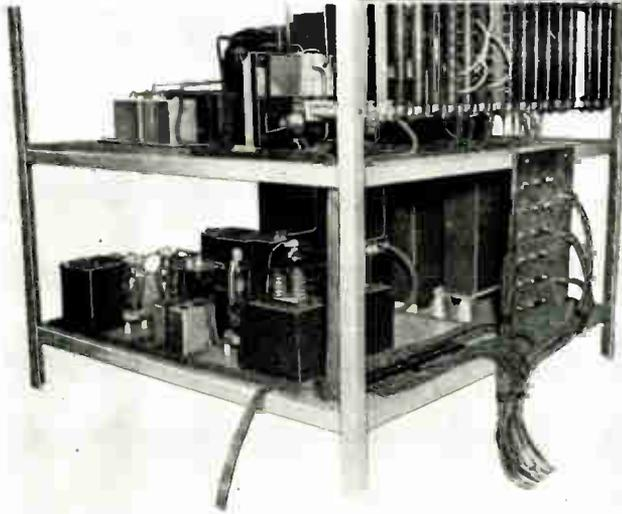
◄ On the bottom shelf of the rectifier are found the high voltage filter capacitors and the low voltage rectifier.
