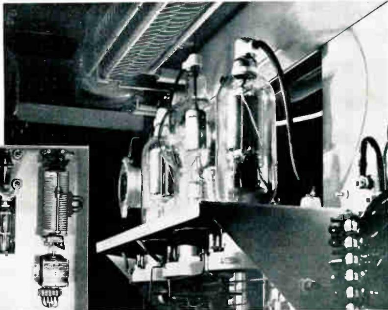
The final amplifier and modulators are shown in the illustration above. A single type 806 or 250TH may be used for the final amplifier without making any mechanical or electrical changes. The modulators are 810 tubes.
