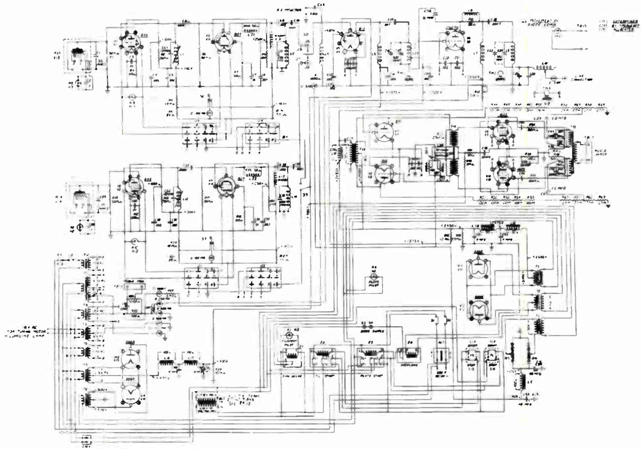
Schematic diagram of the BC-250D.
