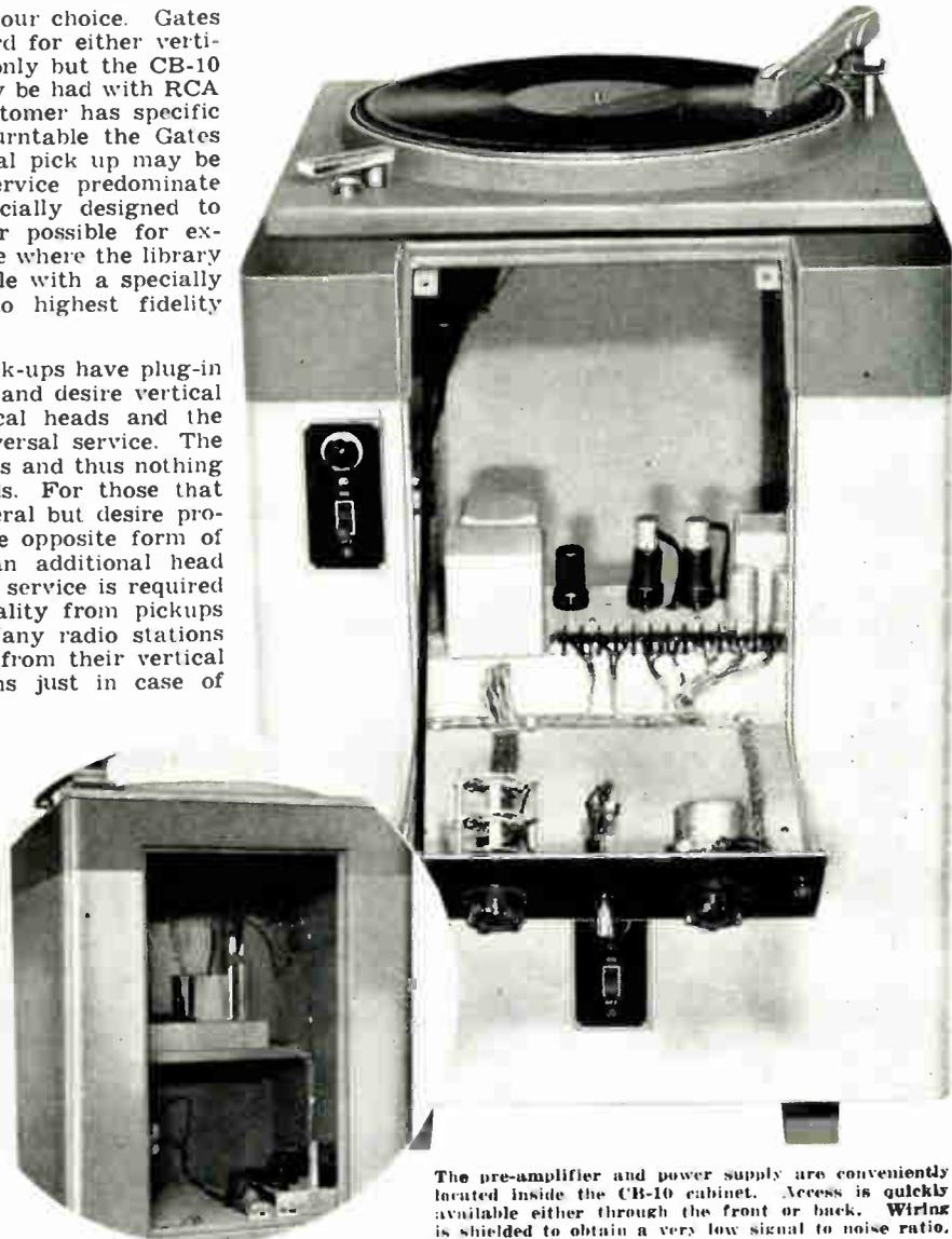
The pre-amplifier and power supply are conveniently located inside the CB-10 cabinet. Access is quickly available either through the front or back. Wiring is shielded to obtain a very low signal to noise ratio.
