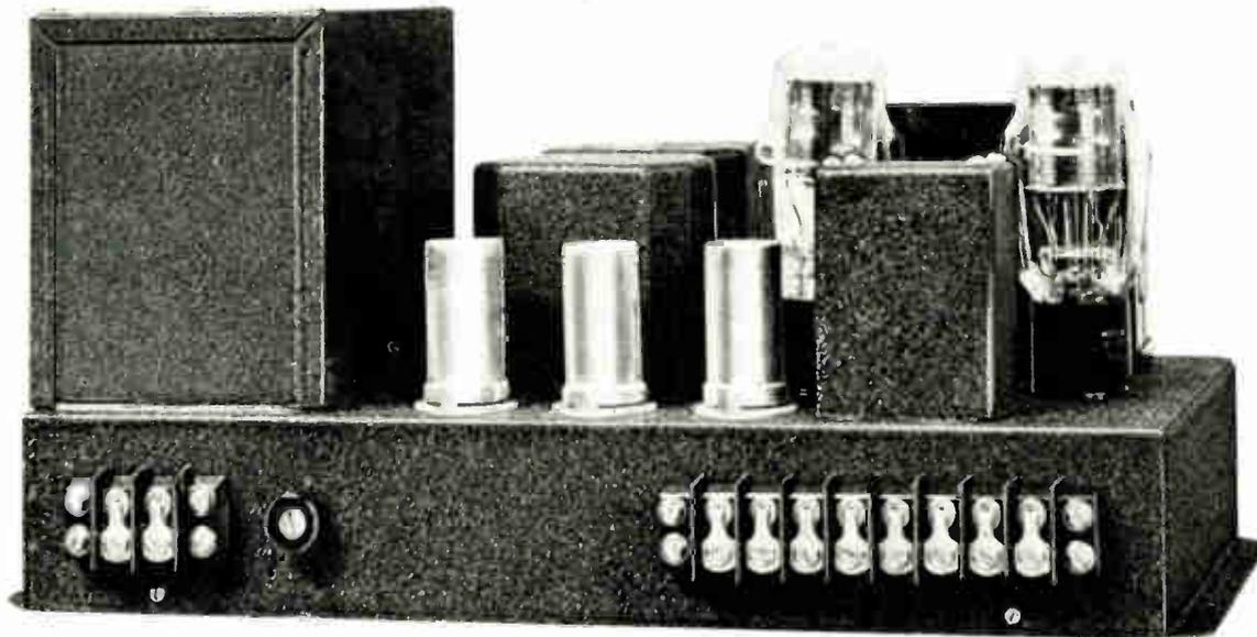
This is the power supply and monitoring amplifier chassis of the Studioette.
