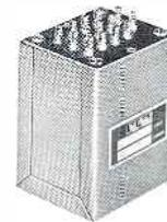
MODEL LE-1: Shown to left is a fixed equalizer. A parallel resonant circuit operating with either a 150 or 600 ohm line. Equalization is varied by means of self-contained resistors in 1 ohm steps up to 111 ohms. Inductance is tuned by 0.05 mfd. and 0.025 capacitors, also self-contained.
