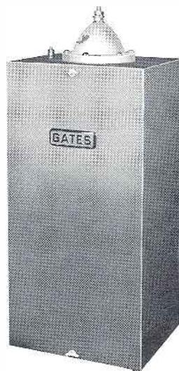
**Model M-5178:** Series feed, provides all coil capacitance to provide full Tee network. Constructed in non-weatherproof steel cabinet, front removable. Size: 21" high, 10" wide, 9" deep. Matches RF input of 50 or 70 ohms. Output 10-600 ohms. In this model metering is external to the coupler, often desirable in unattended operation. For all powers 100% modulated up to 1250 watts carrier.
