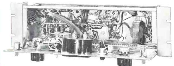
Front panel drops down for complete inner servicing. Big advantage of this type of construction is ability to keep important inner workings clean by means of bellows or small suction type cleaner.
