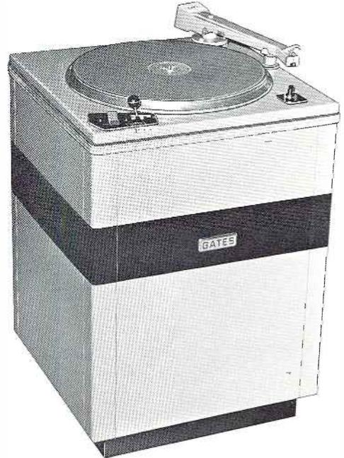
CB-510 complete operating transcription turntable includes CB-500 low noise chassis with synchronous motor, GRAY 208-S/G viscous damped pickup arm, twin flip-over 1 mil and 3 mil reluctance cartridge, 2-position variable equalizer to NAB/RIAA and high frequency roll off curves and M-6244 transistorized preamplifier with self-contained power supply. Output: 150 or 600 ohms adjustable from -22 dbm to -12 dbm, 12 MV input.
