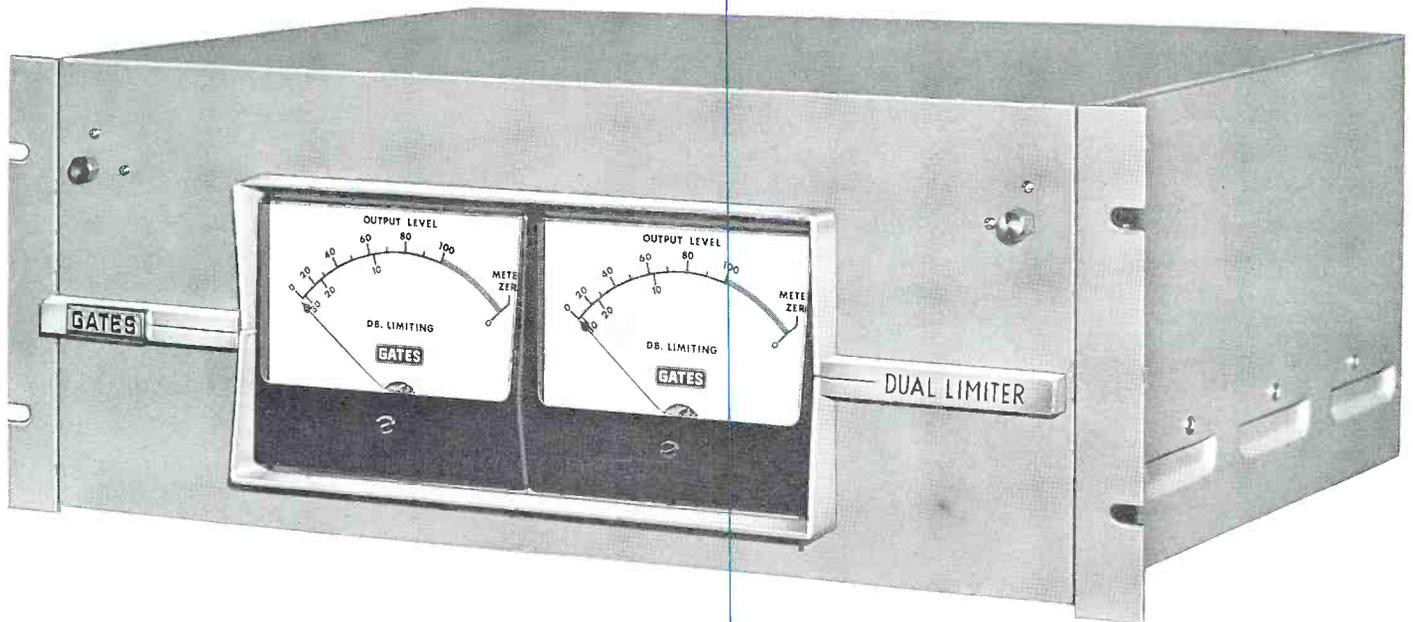
FM stereo broadcasting has created the need for specialized audio equipment. Of major importance is the stereo limiting amplifier. The content of a stereo signal is such that two individual single channel limiting amplifiers will not provide best service. The difference in level between stereo channels may cause one channel to limit heavily while the other is not limiting at all. This will cause unbalance between channels and serious loss of stereo effect.
