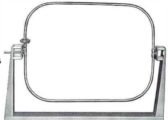
M-3283: This model especially applicable where high current ratios are to be sampled. May be rotated so that phase monitor amplitude values are nearly equal. Electrostatically shielded and insulated from tower. May be used with or without isolation coil at base of tower. Coil is single loop of 7/8" coaxial cable, heavily insulated from base frame. Matches either 50 or 70 ohm line. Size: 48" wide, 32" high.
