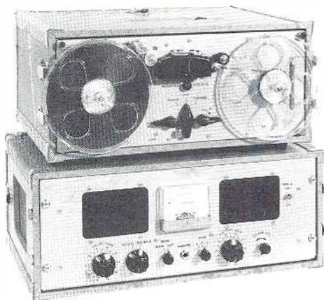
response is from 50 to 15,000 cycles  $\pm 2$  db at 15 ips.
