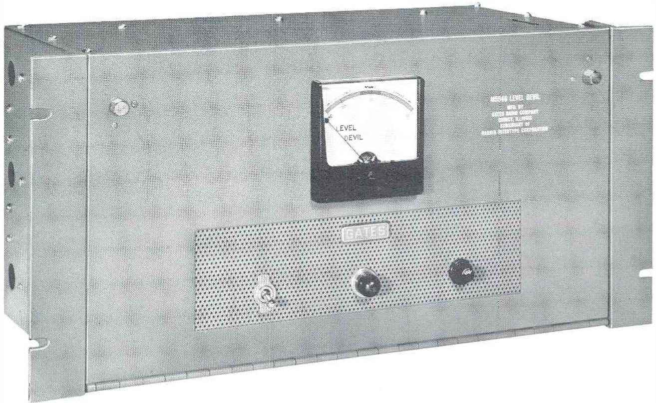
"Level Devil" accepts input signals over a 30 db range and holds the output constant (0 to +3 db). The expander threshold is -10 db relative, and below this the "Level Devil" is a linear amplifier. At this level the gain increases 10 db, and above it the amplifier acts as a peak limiter.
