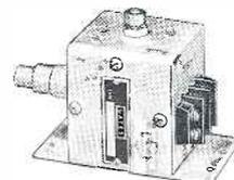
Designed to sample the 51.5 ohm transmission line of an FM transmitter for measuring transmitter output as required by FCC. Provides a DC voltage which is measured on the studio unit meter system. Solid state device requires no AC power.
