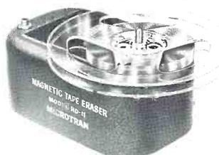
Bulk tape demagnetizer developing high intensity magnetic field. Erases recorded signals and noise completely and restores tape to like new condition. Handles 5", 7" and 10 1/2" reels. Adapter hub available (optional accessory) for 10 1/2" reels. 117 volts, 50/60 cycles.
