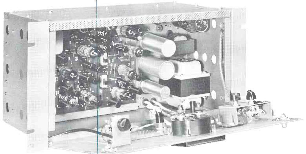
Hinged-down front panel permits complete front accessibility of components and inner servicing adjustments. Printed wiring by the Gates solid adhesion process assures uniformity and ease in both cleaning and circuit analysis. "Level Devil" finish is a medium gloss gray over a heavy prime coat. Design is for continuous duty.
