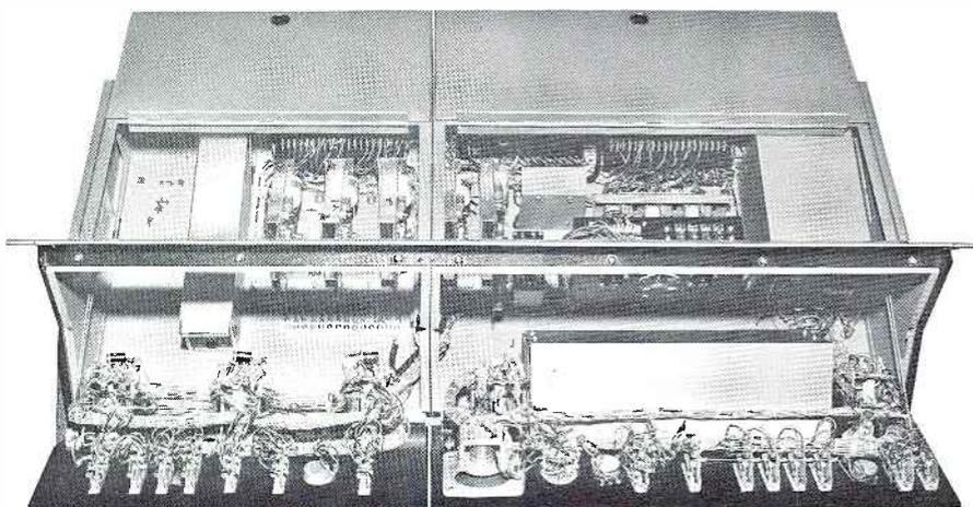
The regulated power supply protects the console amplifiers from variations due to line and load regulation. In addition, the power supply ripple is reduced to the point of nonexistence to assure uniformly low noise in all of the console circuits. The power supply is also short-circuit protected to prevent damage to any of the transistors in either the power supply or amplifiers from a momentary or sustained short in any of the circuits.
