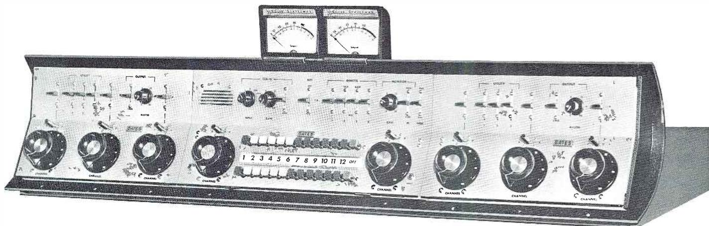
The *President* is a completely transistorized dual channel audio control console, providing eight input mixing channels. It is distinctively designed with a totally new 12-position control center—activated by an array of 24 illuminated touch-control keys for precise fingertip command of input circuits. Twenty-eight inputs are provided in the *President*. When all six of the 3-position utility switches are used to expand the input facilities, a total of 45 inputs are available.
