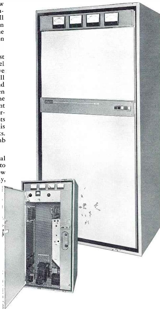
reduces power to 250 watts. Switching in the primary of the main plate transformer eliminates power consuming and heat generating voltage dropping resistors. Plate voltage is reduced on both the power amplifier and modulator tubes, resulting in possible hundreds of added tube hours as well as savings in power costs.
