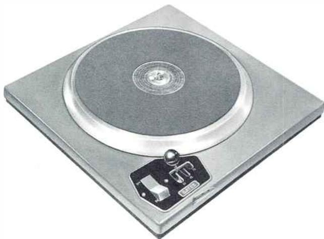
**MODEL CB-77:** Chassis only, ready to attach pickup arm of your choice. For 33 1/3, 45 and 78 RPM with fast pickup-to-speed and low -45 db rumble at 33 1/3 and 45 RPM. Incorporates hysteresis synchronous motor.
