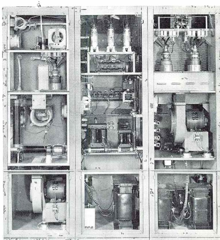
**REMOTE CONTROL:** The exclusive use of relays in the control circuits makes installation of remote control simple. Circuits to be remote controlled are provided with extra terminals.
