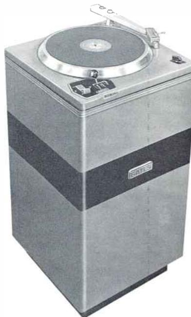
**MODEL CAB-8 CABINET:** Designed to house the CB-77 chassis or CB-88 complete turntables. 16 1/8" wide, 16 1/8" deep and 30" high with leveling screws. Over-all maximum height with chassis mounted is 32 3/8". Built of cabinet maker's birch with corner supports of steel and finished in two-tone gray and black. Back door removable for servicing.
