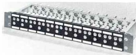
For patching coaxial circuits. 12 groups of 3 jacks on a strip 2 1/8" x 19". Contacts heat treated beryllium copper. Outer braid of coaxial cable may be soldered directly to jacks for complete shielding. Patch cords and plugs listed and illustrated below.
