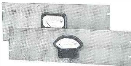
Several types available as listed below for extending both frequency and modulation monitors. Mounted on standard 19" rack panel 5 1/4" high.
