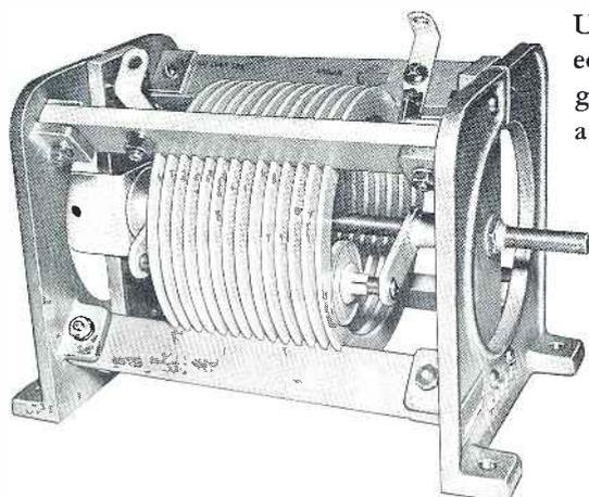
Used in both Gates and many other makes of transmitters and phasing equipment. Variable coils have cast aluminum end bells with double gripping bearing wheels. All types are micaex insulated and silver plated and have the highest possible "Q's".
