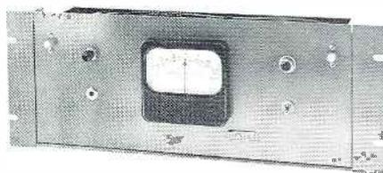
Used for extending Gates M-2890 monitors. Has 4" frequency indicating meter reading 30-0-30 cycles. Includes resistor pad for sampling voltage. Tubes: 6AW6, 6AQ5, 6AL5, 6X4 and OA2. For 115 volts, 50/60 cycles.
