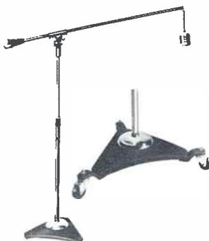
Boom length 62" (more extension addable). Adjustable vertical extension 48"-72". Base diameter 17". Tubular sections superchrome plated. Modernistic base finished in chrome and gun metal shrivel. "Snap On" hangers furnished to hold mike cable to boom section. Ship. Wt. 33 lbs.
