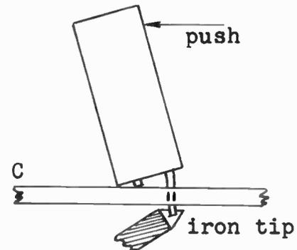
(A) hold iron tip on one of the folded leads, as soon as the solder melts - push gently but firmly on the side that will lift this lead. The capacitor should be pushed over just far enough to clear the lead from the hole.
