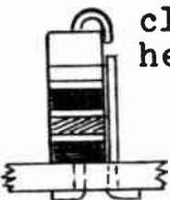
B pliers place iron on fillet and push wire through the hole until the hook can be clipped off.
