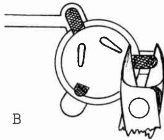
Using a pair of small sharp diagonal cutters, bend the mounting ears up and away from the copper conductor pads. DO NOT PRY THE MOUNTING EARS UP WITH A KNIFE OR SCREWDRIVER!
