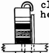
clip here B
