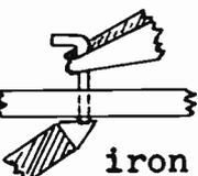
pliers clip off hook that was soldered to chassis.
