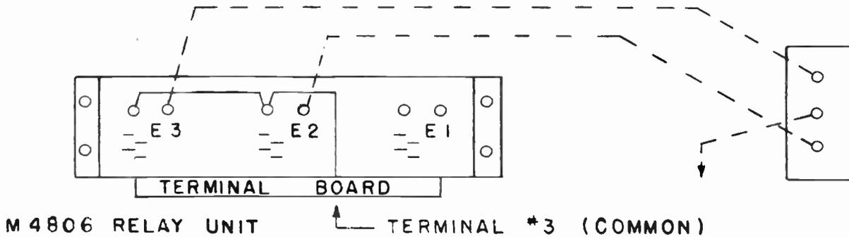
Solder two leads to A.C. relay terminals opposite common connection, and connect to two outside terminals of motor switch.
