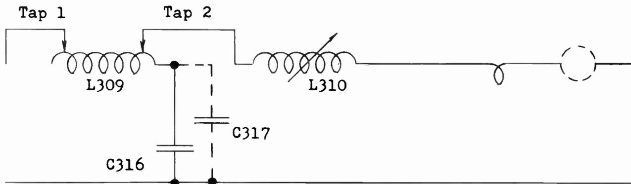
Tap 2 is adjusted so that the inductance between this tap and the end of the coil connecting to the coupling condensers, with the coupling condensers C316/317 form a series resonance circuit at the unwanted frequency. The position of tap 2 may be critical to  $1/4"$ . The normal loading is then adjusted by the position of tap 1. This circuit shows 10 to 20 DB attenuation to the undesired signal.
