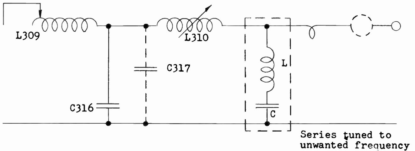
The condenser C can be the same type and capacity as at C316/C317. The circuit is tuned to normal loading on the fundamental without L. The coil L is tuned to the unwanted frequency when connected in parallel to C, using a grid dip meter. The coil L should be of 1/4" or 5/16" copper tubing. The mounting should be for minimum coupling to other circuit elements. With careful adjustment 20 to 30 DB attenuation may be obtained.
