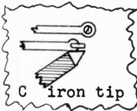
place the iron against the folded wire and rotate it away from the conductor leading into the fillet (2-c).
