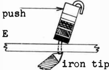
place iron on fillet again and push the resistor body over until the lead comes out of the hole.
