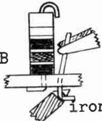
iron tip clip off hook that was soldered to chassis.
