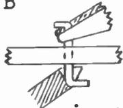
iron tip clip off hook that was soldered to chassis.
