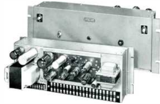
Two Rack Mounted Monitor Amplifier Supply Assemblies are included as standard equipment.
