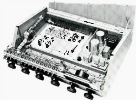
Hinged top cover and front panel swing open for easy access to components.
