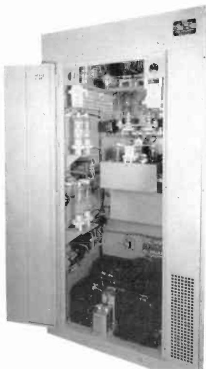
These two rear views of the HF1 transmitter picture the left section of radio frequency portion. The engineer will note the symmetrical design which assures perfect circuit balance, necessary for high efficiency and stability.
