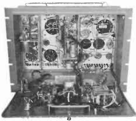
To service equipment mounted on SA housings, drop down the rigid cast front door. Note how every under-chassis component can be reached. Cabinet style strips need not be removed to drop down front door.
