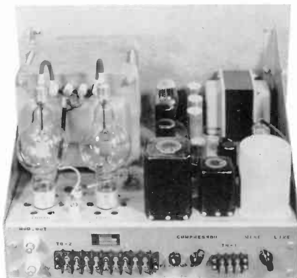
Left, below, is complete radio frequency chassis of CMW-1 transmitter. Right, below, is the speech amplifier-modulator unit with self-contained limiter and 3000 cycle cutoff filter.
