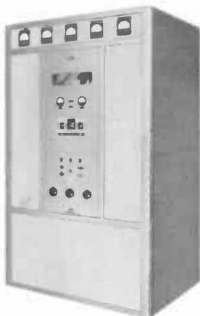
For heavy duty service, the Gates 1000-watt amplifier stands 78" high, 40" wide and 36" deep. Operates from 220 volts single phase.
