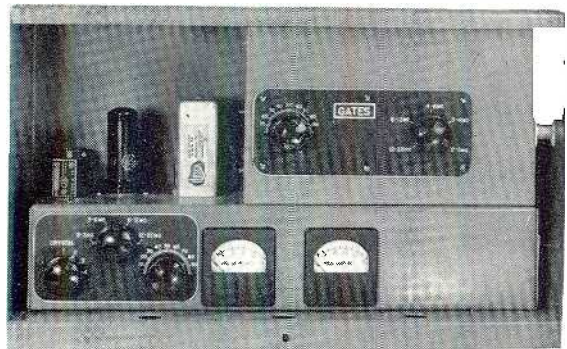
Front view of the oscillator-buffer section removed from transmitter. One of four crystals may be selected, and may be either temperature or non-temperature controlled.
