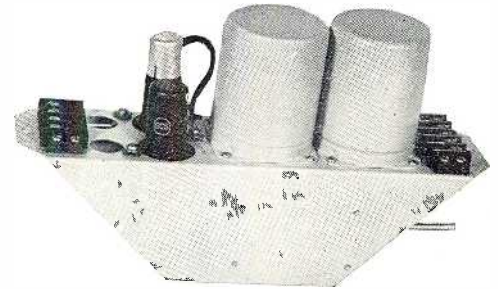
Figure A—The SA-70 preamplifier. The gain control included allows any gain adjustment. Tubes are shock mounted.
