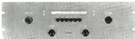
Remote unit provides complete control of the CMP-1 transmitter from operator's desk. The remote panel is an accessory item.
