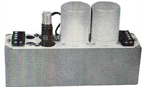
Figure B—The SA-71 preamplifier in housing for turntable cabinet mounting or similar application. Mounting holes are provided in bottom of housing.
