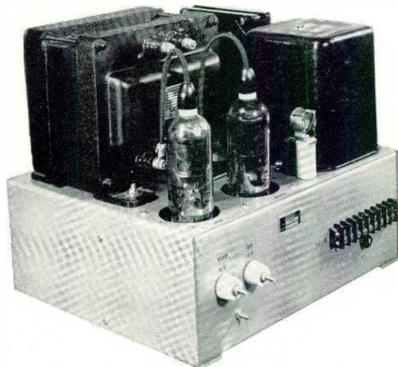
Above, left, the low voltage power supply deck. Right, the main high voltage supply delivering 2300 volts to power amplifiers and modulators.
