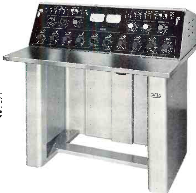
This front view, with panel dropped down, illustrates inner terminal arrangement for attaching external patch panel, where desired. The patch panel is not by any means a necessity in the console operation.
