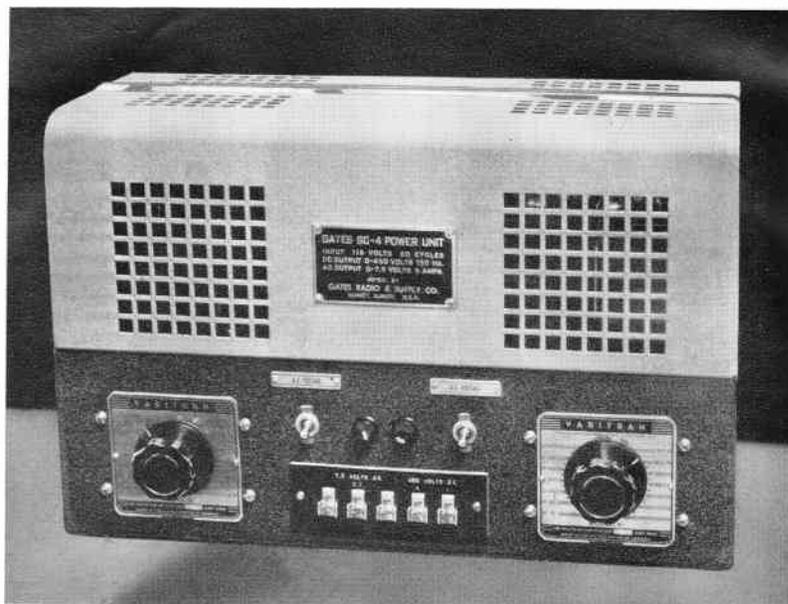
Above is illustrated the SC4 power unit which is available in numerous AC and DC voltages. The unit illustrated developed 450 volts at 150 Ma. D. C. at less than .25% ripple content and is variable from 0 to maximum voltage by means of an auto transformer. A. C. voltage is 7.5 volts maximum with exact center tap and is variable also from 0 to full voltage providing tests on common tube voltages of 1.1, 2, 2.5, 5, 6.3 and 7.5 volts. An extremely handy unit for production or test bench service.
