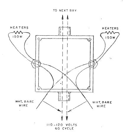
The two bare wires indicated extending from the junction box are to be connected parallel across the 110-120 volt line. In checking for continuity of heaters, any reliable multimeter that will measure between 0-100 ohms will be sufficient. Single heaters should measure 75 ohms, two in parallel will be half of this, approximately 37 ohms.
