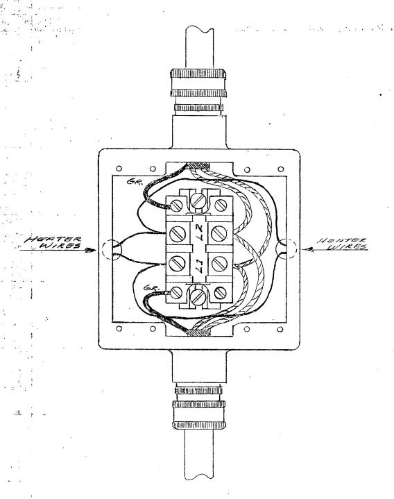
Remove male portion of connectors from cable and screw into junction box.
