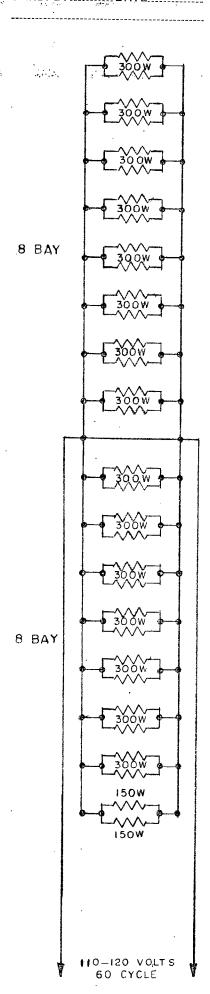
300 Watt Heaters Each Element rated 150 Watts at 120 V
