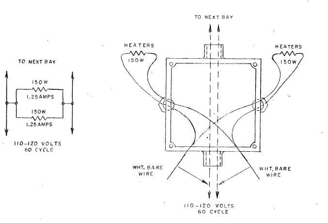
The two bare wires indicated extending from the junction box are to be connected parallel across the 110-120 volt line. In checking for continuity of heaters, any reliable multimeter that will measure between 0-100 ohms will be sufficient. Single heaters should measure 75 ohms, two in parallel will be half of this, approximately 37 ohms.
