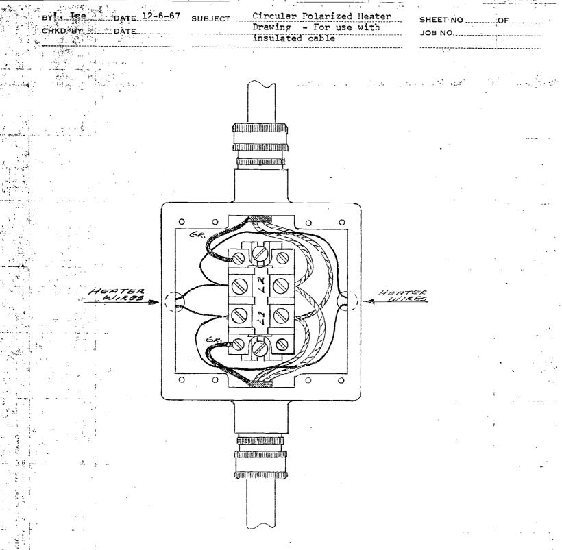
Remove male portion of connectors from cable and screw into junction box.
