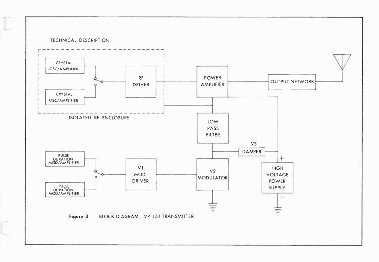
The modulator, V2, is connected through a low pass filter to the cathode of the power amplifier. The low pass filter provides the necessary function of removing the 70 kHz frequency component and the harmonics thereof and of recovering the audio as a modulating signal for the power amplifier. Note that the modulator is in series with the power amplifier.
