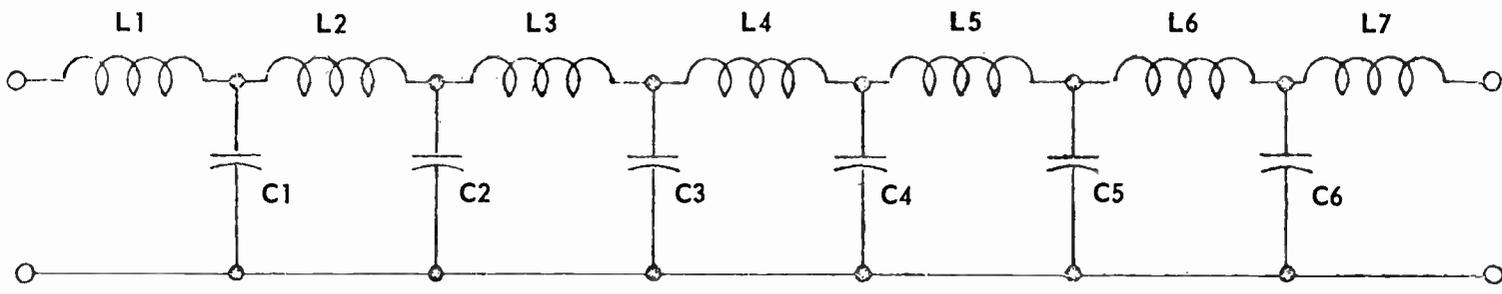
EQUIVALENT CIRCUIT - LOW PASS FILTER
