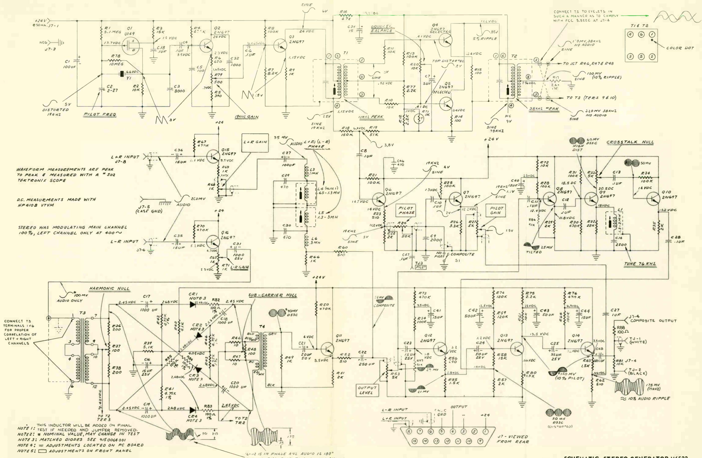
WAVEFORM MEASUREMENTS ARE PEAK TO PEAK & MEASURED WITH A #502 TEKTRONIX SCOPE
