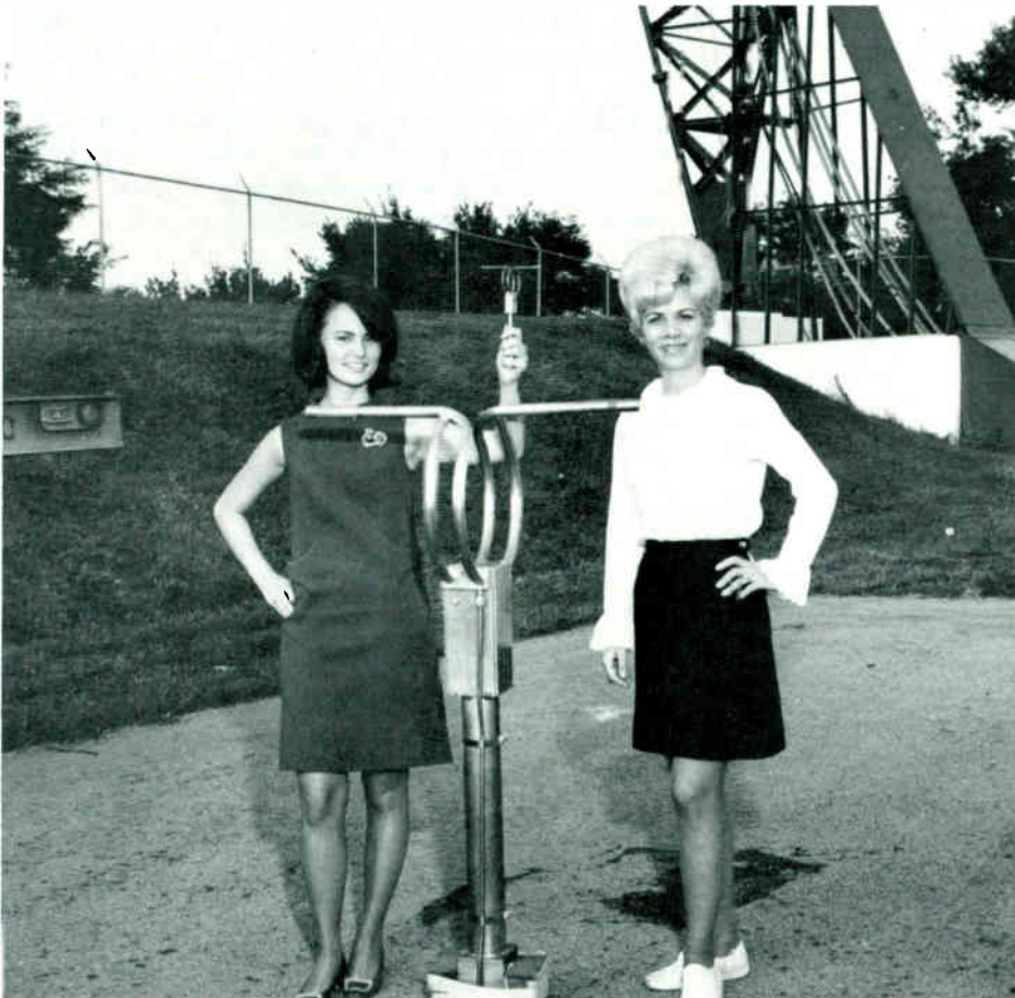
Models hold one element of the Gates' Dual Cycloid circularly polarized antenna which is now mounted atop the antenna tower at station WSM-FM, Nashville, Tenn. The antenna installation consists of 14-bays.
