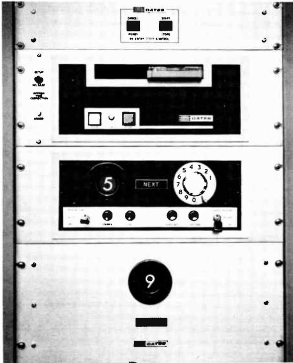
The SP-10 and SP-19 program control systems provide fully automatic control of audio automation systems. The SP-10 unit will function with up to 10 audio sources, and as many as 19 may be controlled with the SP-19 Programmer.
