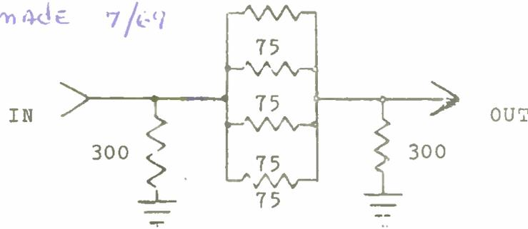
The 3 dB isolation network is contained in a 1-5/8" x 2-1/4" x 2-3/4" aluminum box mounted inside the transmitter cabinet directly behind the TE-1 output connector.
