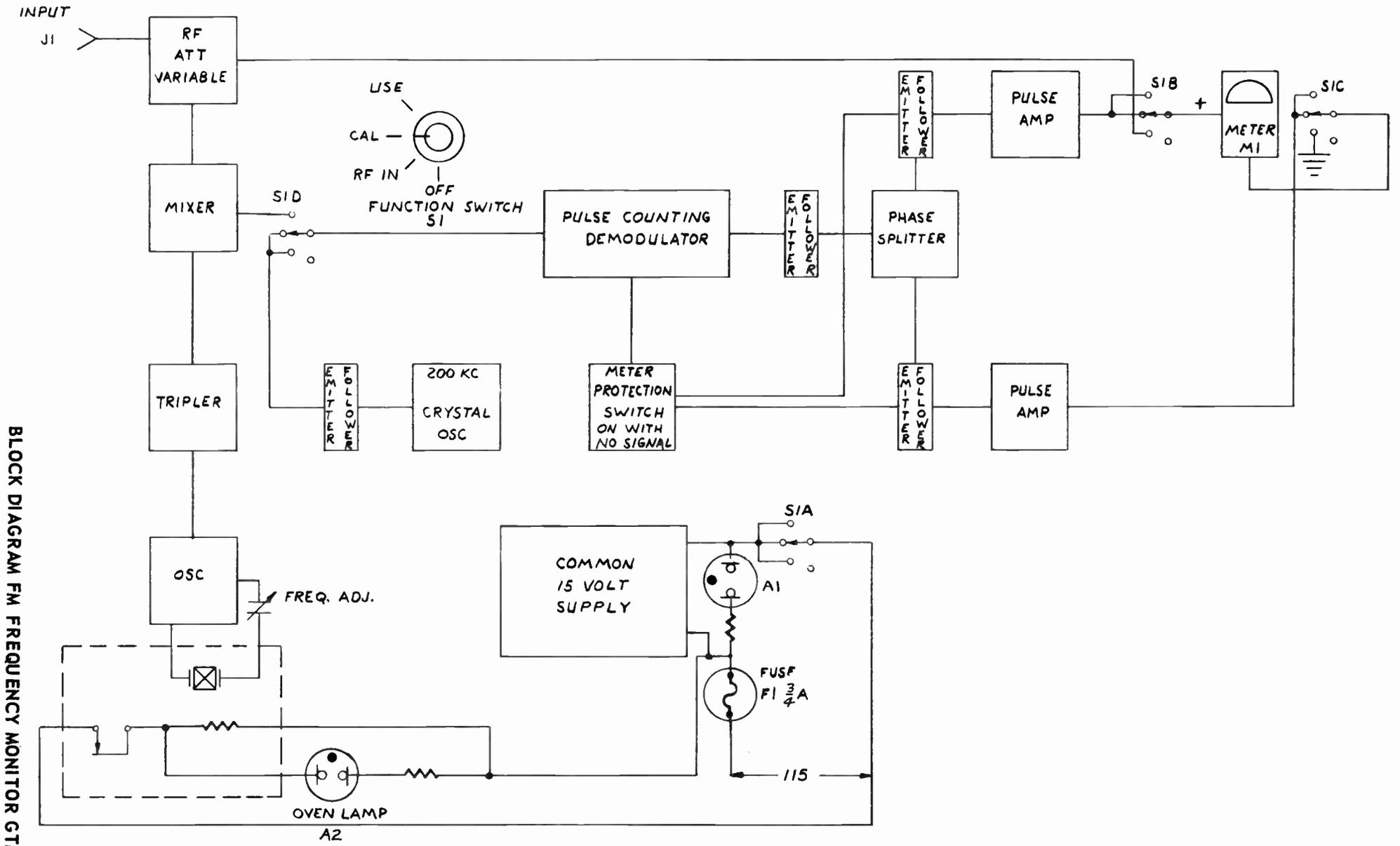
BLOCK DIAGRAM FM FREQUENCY MONITOR GTM-88F
