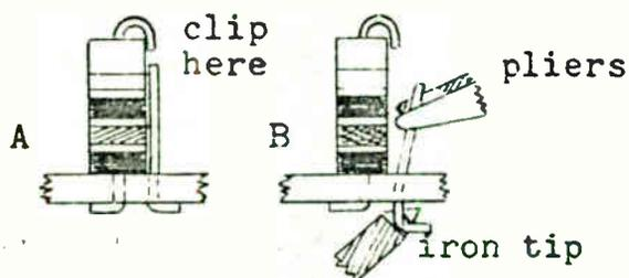
Fig. 9 - Removing Components
