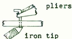
Fig. 8 - Removing Lead
