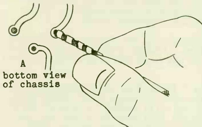
Use a small metal twist drill (1/8" dia. or less) to clear the hole only in the fillet of solder. Twirl the drill by hand. Do not attempt to remove all of the solder in one turn, do it slowly and carefully.
