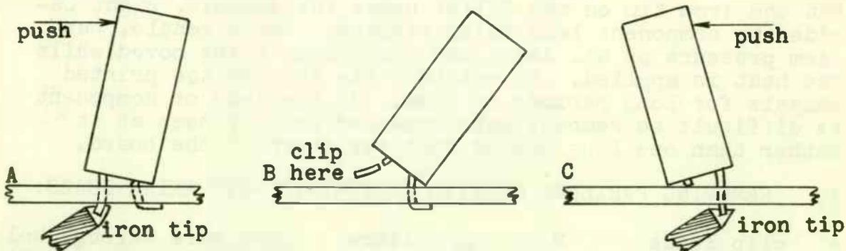
(A) hold iron tip on one of the folded leads, as soon as the solder melts - push gently but firmly on the side that will lift this lead. The capacitor should be pushed over just far enough to clear the lead from the hole.
