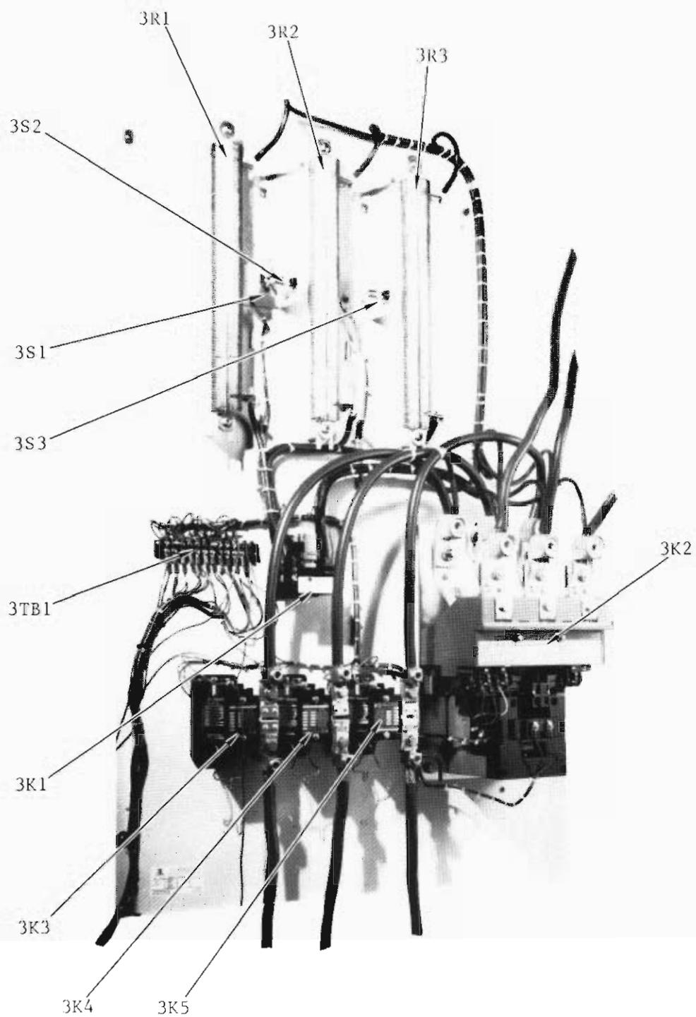
Figure 2-16. High-Voltage Step-Start Assembly
