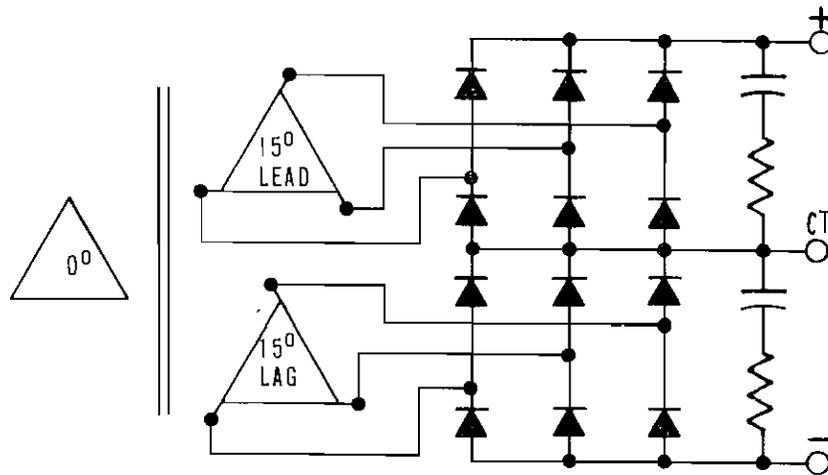
Figure 4-5. 12-Phase Circuit
