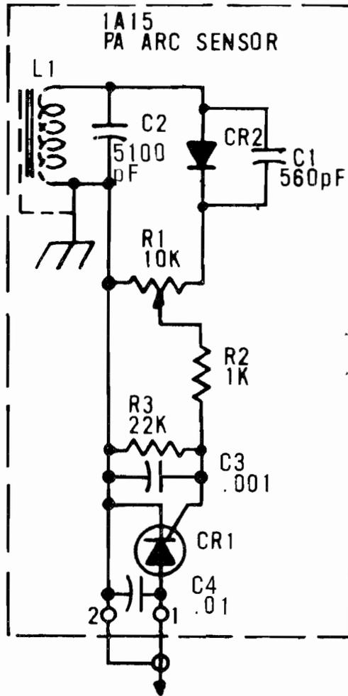
FIGURE 9-9. PA ARC DETECTOR
