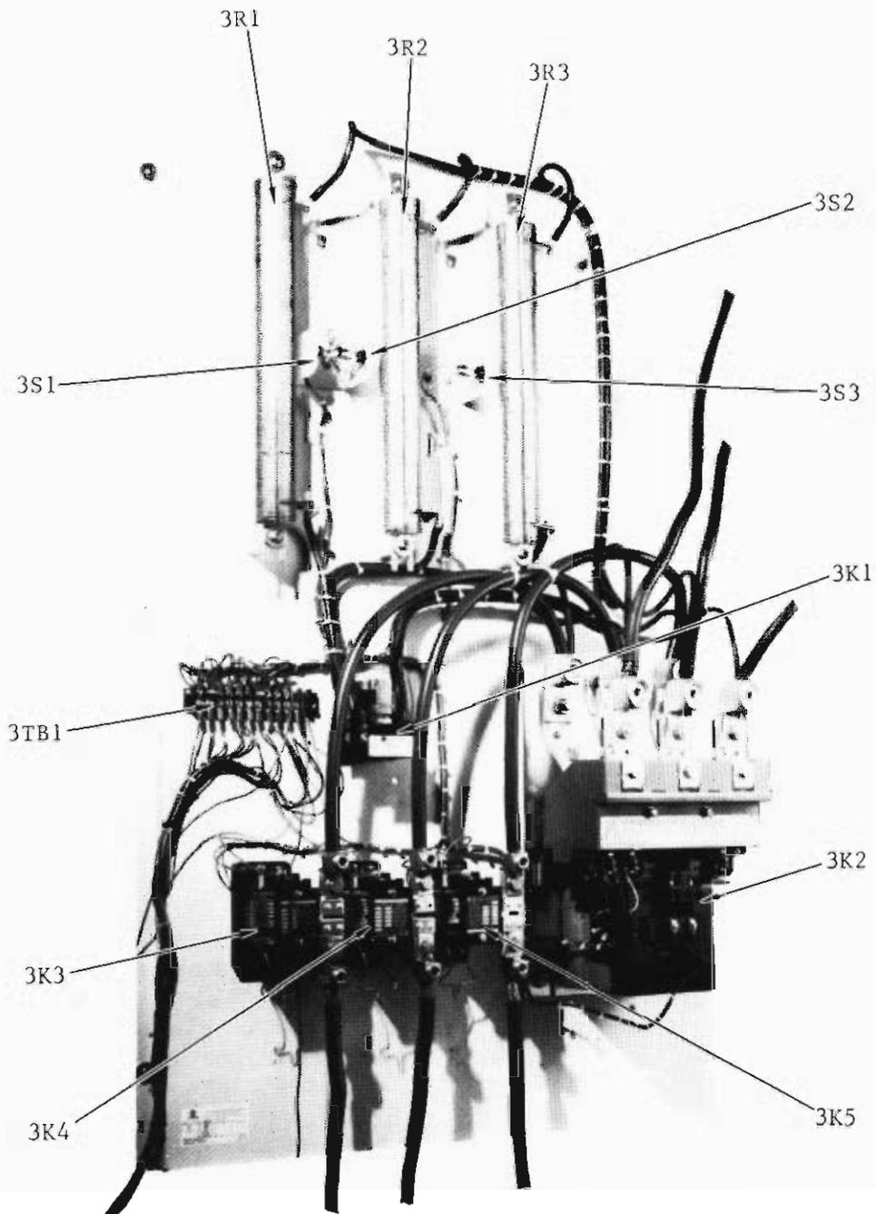
Figure 1-2. High-Voltage Step/Start Assembly
