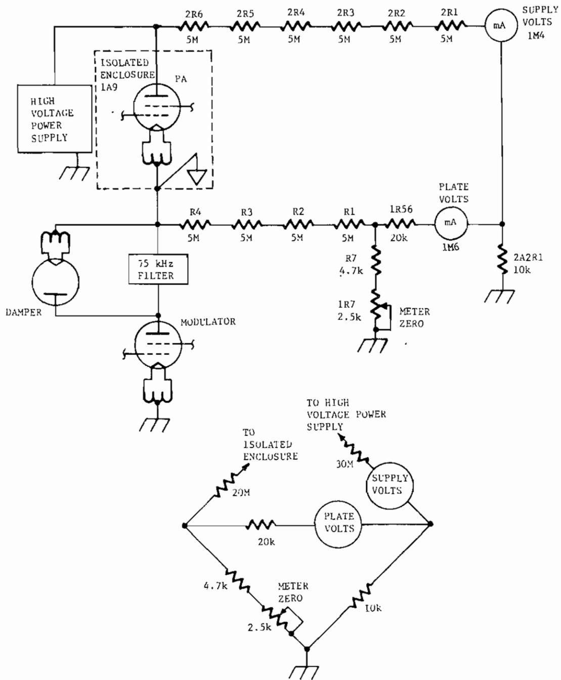
Figure 4-11. High Voltage Metering
