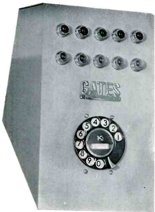
FIGURE A —Illustrates above the desk type dial circuit selector. This houses the dialing unit, circuit indicating lights and terminal connections which operate the stepping and control relays mounted on a separate rack panel. Its small size of 6\frac{3}{4} inches wide and 10\frac{1}{2} inches high makes it convenient for any type of desk mounting.
