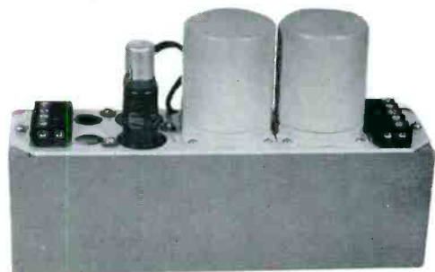
Figure B—The SA-71 and SA-74 preamplifiers in housing for turntable cabinet mounting or similar application. Mounting holes are provided in bottom of housing.
