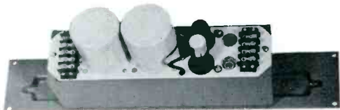
Figure D—Back view of SA-72 or SA-75 rack mount preamplifiers. Note the shock mounting of tubes, test jacks for plate current, metering and isolation of input and output terminations.
