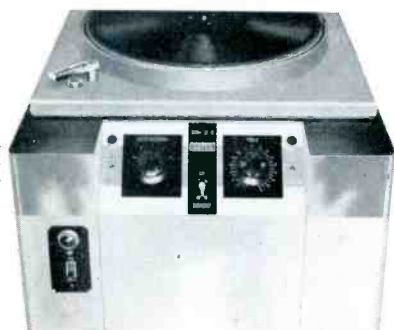
Figure B—The front section drops down for instantaneous accessibility of preamplifier and power supply tubes.
