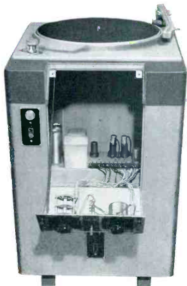
Figure B—The front section drops down for instantaneous accessibility of preamplifier and power supply tubes.
