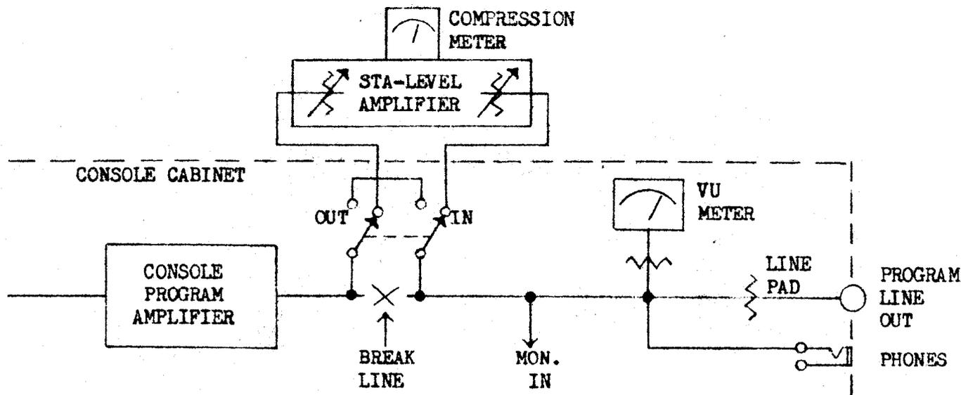
Almost any console is easily modified for use with Gates' STA-LEVEL Amplifier as shown above. Simply remove the output from the console program amplifier, as shown by the break, and connect to the input terminals of the STA-LEVEL Amplifier. Connect the output of the STA-LEVEL Amplifier to the output circuit of the console. The use of a console utility switch, or an external switch, will allow the STA-LEVEL Amplifier to be switched in or out of the circuit as desired.
