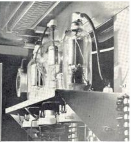
The final amplifier and modulators are in the illustration above. A single type 450TH or 250TH may be used for the final amplifier without making any mechanical or electrical changes. The modulators are 813 tubes.
