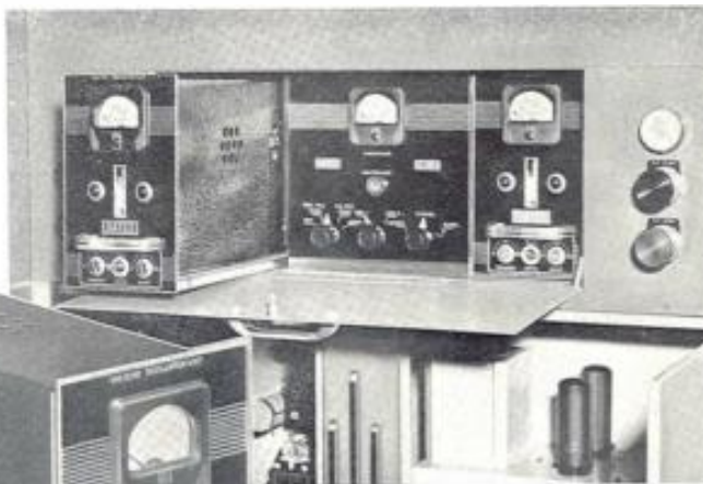
Above is the "Customaire" showing front doors open and wide accessibility to tubes and relays. At the right is a close-up of the frequency control unit section. On the center panel are the tuning controls for the entire transmitter.
