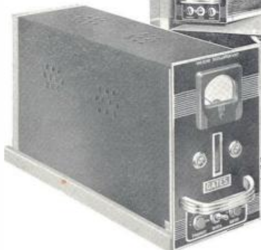
At the left is shown one of the frequency control units removed from the transmitter. Each one contains a complete oscillator and first buffer with crystal and oven. The thermometer on the crystal oven can be viewed through the vertical slot on the front. Tuning controls and switch for changing the meter from the plate circuit of the oscillator to that of the buffer are located at the bottom of the panel.
