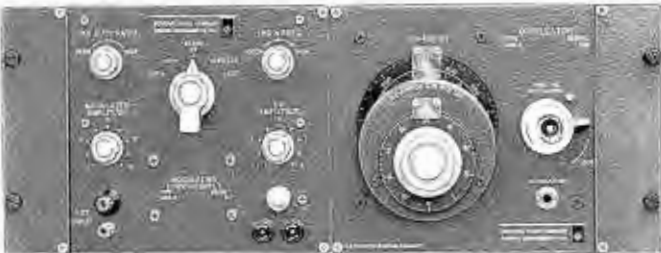
The Type 1361-A UHF Oscillator and Type 1264-A Modulating Power Supply assembled with Type 480-P416 Adaptor Plate Set for rack mounting.
