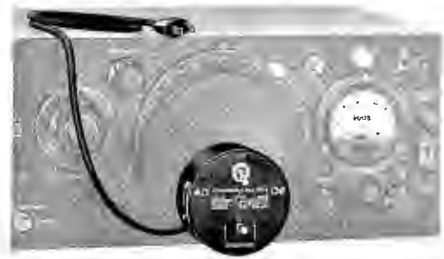
Motor drive attached to a Type 908 dial on the Type 1304-B Beat-Frequency Audio Generator.
