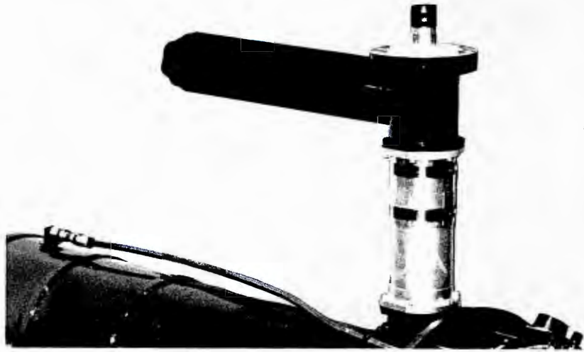
The Variable Visual Coupler employed in the TVE-55 greatly increases the visual klystron's efficiency over the previously used fixed couplers.
