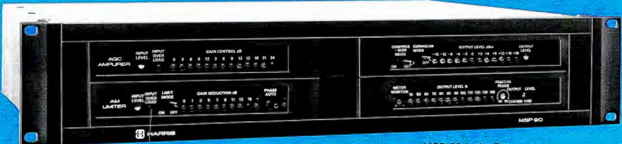
MSP-90 Audio Processor; AGC Amplifier/AM Limiter Configuration
