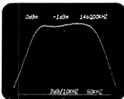
Spectrum analyzer response of Flat-Pass output network maximizes mono and stereo performance.
