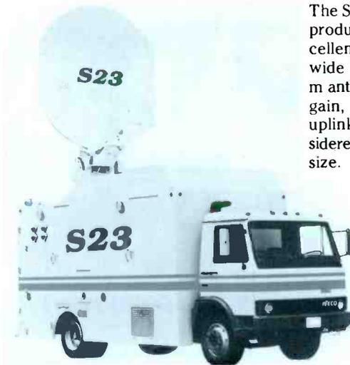
The S-23 is spacious enough for full production capability yet has excellent weight distribution and a wide GVW safety margin. The 2.6 m antenna, with a 50.1 dbi transmit gain, has been field-proven to uplink in areas previously considered impossible for antennas this size.
