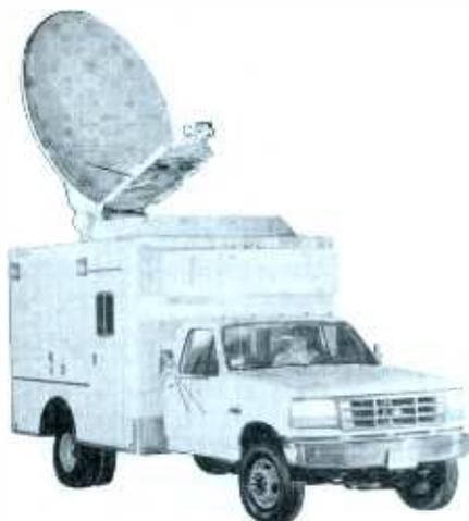
The S-21 is a versatile and compact, heavy duty mobile satellite system. Equipped with its 1.8 m or 2.4 m, high gain, Ku-band antenna, and international power generation system, the S-21 can be adapted for a multitude of uses from spot news coverage or video teleconferencing to data transmission from remote locations. The S-21 combines both flexibility and quality into a compact self-contained, highly mobile unit.
