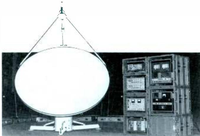
The S-2 "Flyaway" uplink system is the world's premiere high performance, totally "man-portable" C- and Ku-band uplink system. The entire system is packaged in 18 heavy duty aluminum/composite equipment cases, each of which conforms to international baggage size restrictions. The 2.4 meter Vertex antenna in the S-2 has a transmit gain of 49.0 dB and meets or exceeds the 29-25 FCC 2° spacing curves.
