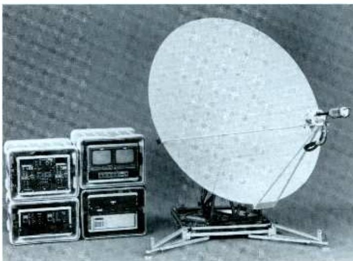
The S-1 'Flyaway' is the world's first high performance, truly portable Ku-band uplink system. It is entirely contained in 14 cases, each weighing less than 100 pounds and conforming to international baggage requirements. The S-1's 1.8M Vertex antenna has a transmit gain of 46.6 dBi and meets the 29-25 ° FCC 2° spacing curves.
