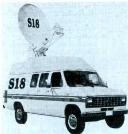
The S-18, a high performance satellite communications system, can maneuver easily in city traffic or on country roads. It uses a Vertex 1.8 m offset-fed antenna with a 46.6 dbi transmit gain for communications flexibility. The S-18 is ideal for uplinking news or special events and is easily adaptable for voice and data applications.
