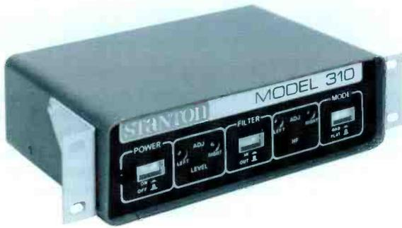
The Stanton 310B preamp features universal mounting by special brackets, instant selection of flat or NAB post-emphasis curves, switchable effective rumble filter, individual adjustment of gains and high frequency responses, trimming of the capacitive cartridge loading at the input and immunity to external magnetic AC fields.
