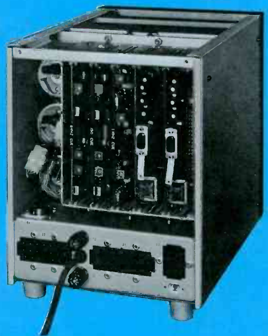
Two Criterion 90-3's may be mounted side by side in a standard rack to provide six playback units in a rack space that will hold only two regular size playbacks.
