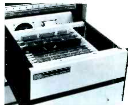
Figure 6: "Slide-out" rack mount chassis provide easy access to all circuitry.
