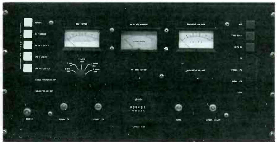
RF monitoring, metering and status light system.
