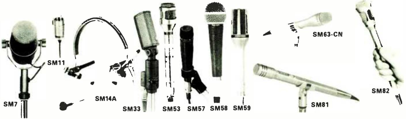
**Model SM7:** A dynamic microphone with a very smooth, flat, wide-range frequency response; cardioid polar pattern, uniform with frequency and symmetrical about the axis; internal "air suspension" shock isolation; highly effective pop filter; extremely good rejection of electro-magnetic hum due to a built-in hum rejection system; bass roll-off and mid-range emphasis. The Model SM7 was field-designed to be the finest dynamic microphone available for music recording and reproduction.
