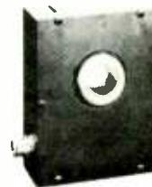
The TCT-1, TCT-2 and TCT-3 are precision toroidal current transformers designed primarily for obtaining sampling voltages for phase and magnitude measurements on broadcast arrays. The units are housed in rectangular aluminum shield enclosures with a 1 1/4" teflon lined pass hole through which the current carrying conductor is passed.
