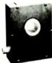
The TCT-1, TCT-2 and TCT-3 are precision toroidal current transformers designed primarily for obtaining sampling voltages for phase and magnitude measurements on broadcast arrays. The units are housed in rectangular aluminum shield enclosures with a 1/4" teflon lined pass hole through which the current carrying conductor is passed.
