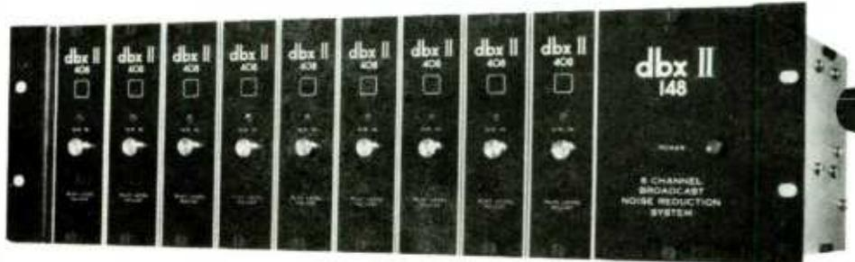
dbx's patented RMS level detector insures perfect decode tracking for accurate transient response despite phase shifts in the transmission or storage medium.
