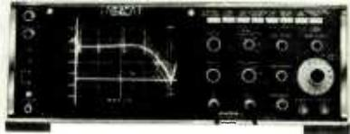
The 201-1 is expressly designed for measuring the envelope delay incurred in equipment used in the transmission and reception of color television signals.
