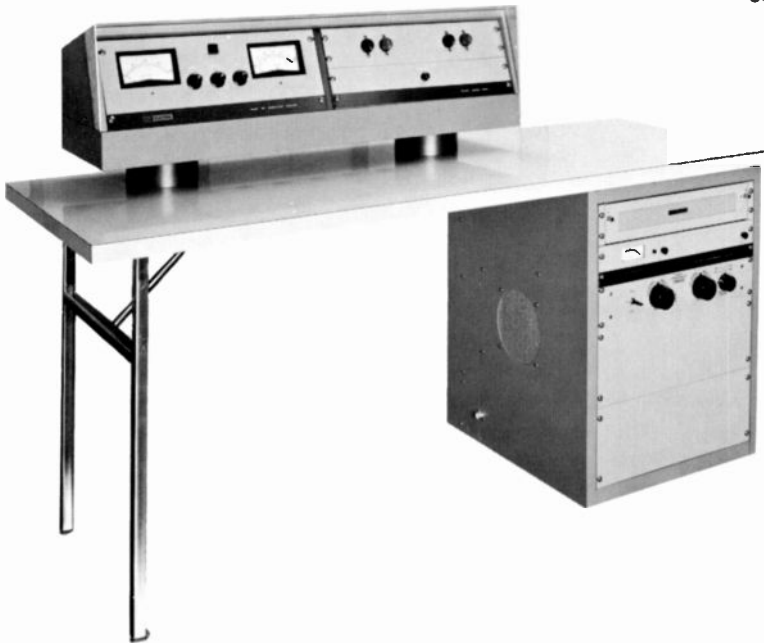
SINGLE TRANSMITTER CONTROL CONSOLE
