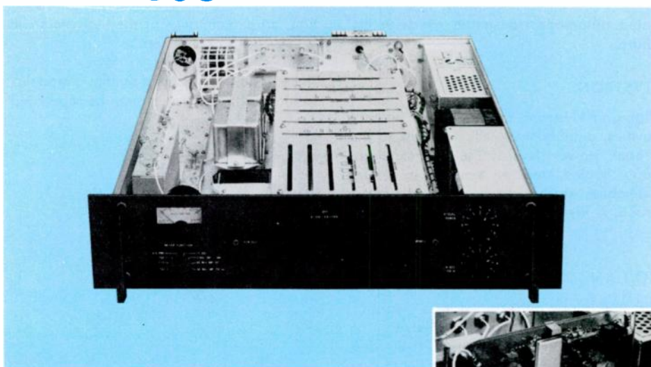
The MCP-1U visual exciter/modulator (above) is a solid-state, independent, self-contained "on-channel" signal source. Harris' advanced TSB filter (right) is mounted on a PC board in the visual exciter, and measures only 1½ inches square.
