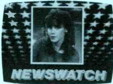
The new image is compressed, given a border, then overlaid upon another existing still that includes a digitally keyed-in title w/drop shadow.
