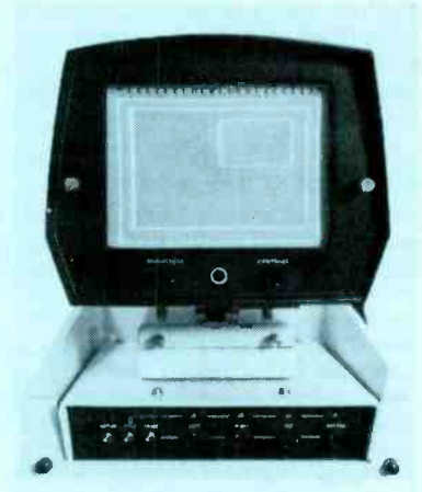
Operator's view of Harris C Series tilttable, rotatable viewfinder showing electronic-generated safe-title area and variable grease pencil window.
