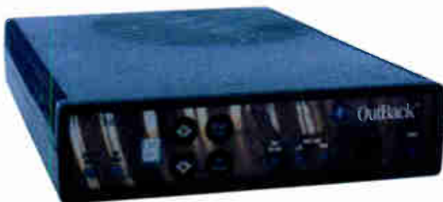
The Harris/Intraplex OutBack (bottom) ISDN codec and the Silence Monitor (top) made by Broadcast Tools can be combined to create a reliable backup for a station's STL. An absence of audio will close a relay in the Silence Monitor and switch the audio feed to a backup link via the OutBack codec and ISDN line.
