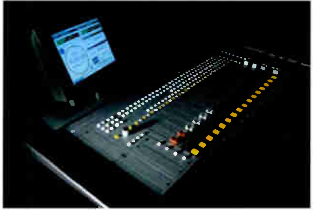
The PR&E Integrity digital console has an ergonomic control surface less than 1.5 inches high. All 16 inputs can handle analog signals. Ten also accept digital inputs at any sample rate.
