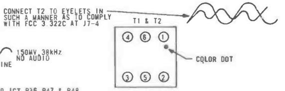
WAVEFORM MEASUREMENTS ARE PEAK TO PEAK & MEASURED WITH A #502 TEKTRONIX SCOPE
