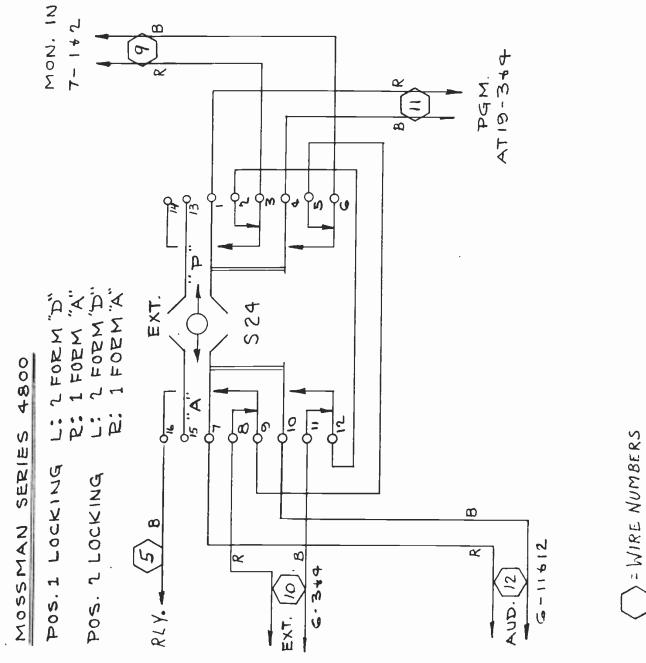
MONITOR IN SWITCH SECTION GATESWAY CONSOLE M5133 811 0996 001
