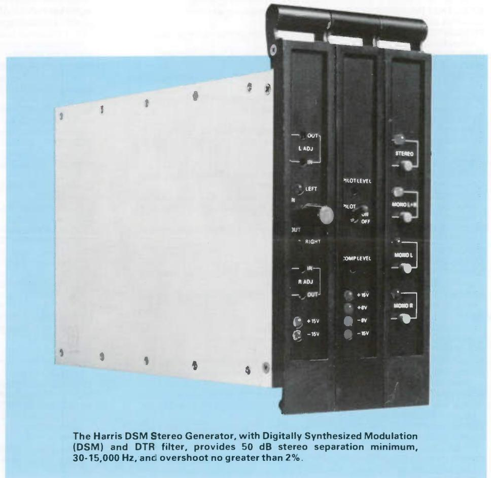
The Harris DSM Stereo Generator, with Digitally Synthesized Modulation (DSM) and DTR filter, provides 50 dB stereo separation minimum, 30-15,000 Hz, and overshoot no greater than 2%.
