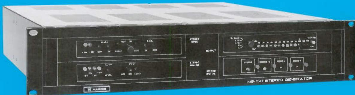
Audio inputs are transformerless and balanced to give maximum common mode rejection while maintaining excellent transient and frequency response. Inputs will withstand high transients or steady state voltages above or below ground level.
