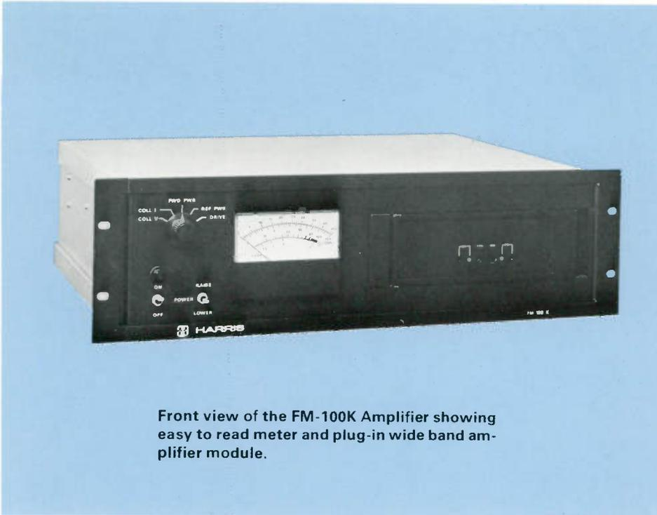
regulator also implements VSWR protection. Should a high antenna VSWR be detected by the built-in directional coupler, the voltage regulator automatically turns down the supply voltage to the amplifier.
