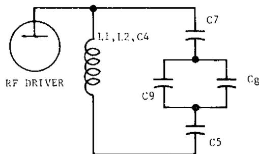
Figure 4-7. RF Driver Plate Circuit
