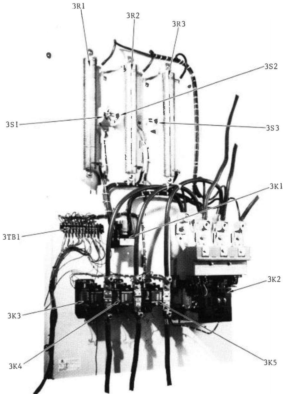
Figure 1-2. High-Voltage Step/Start Assembly
