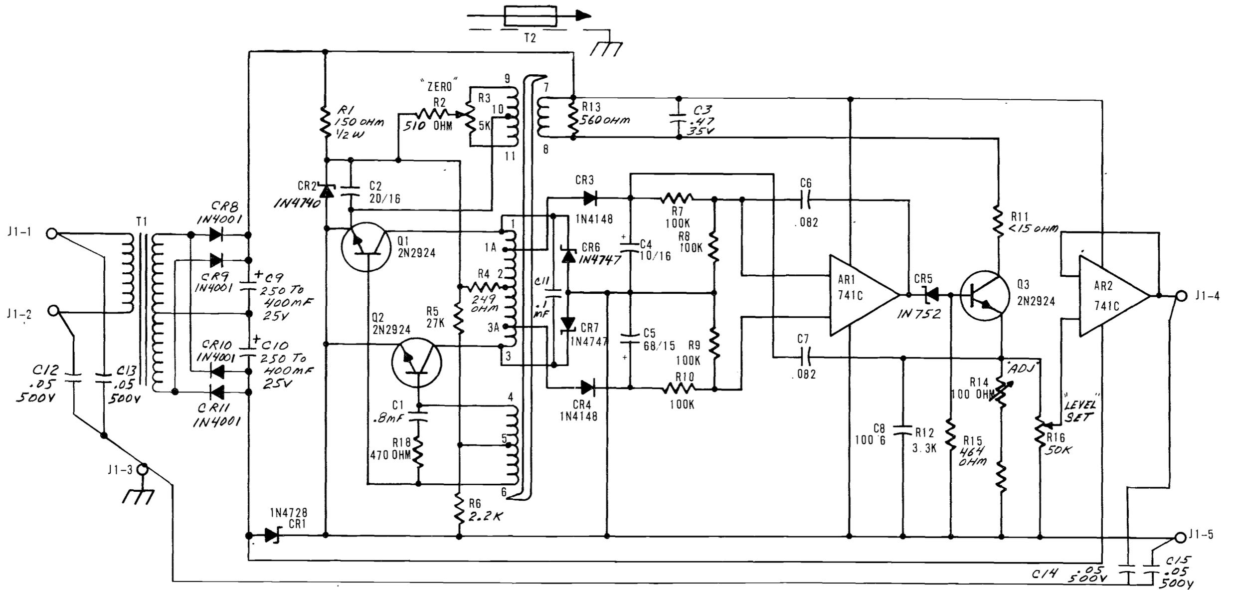
FIGURE 9-8. REMOTE PLATE CURRENT SENSOR
