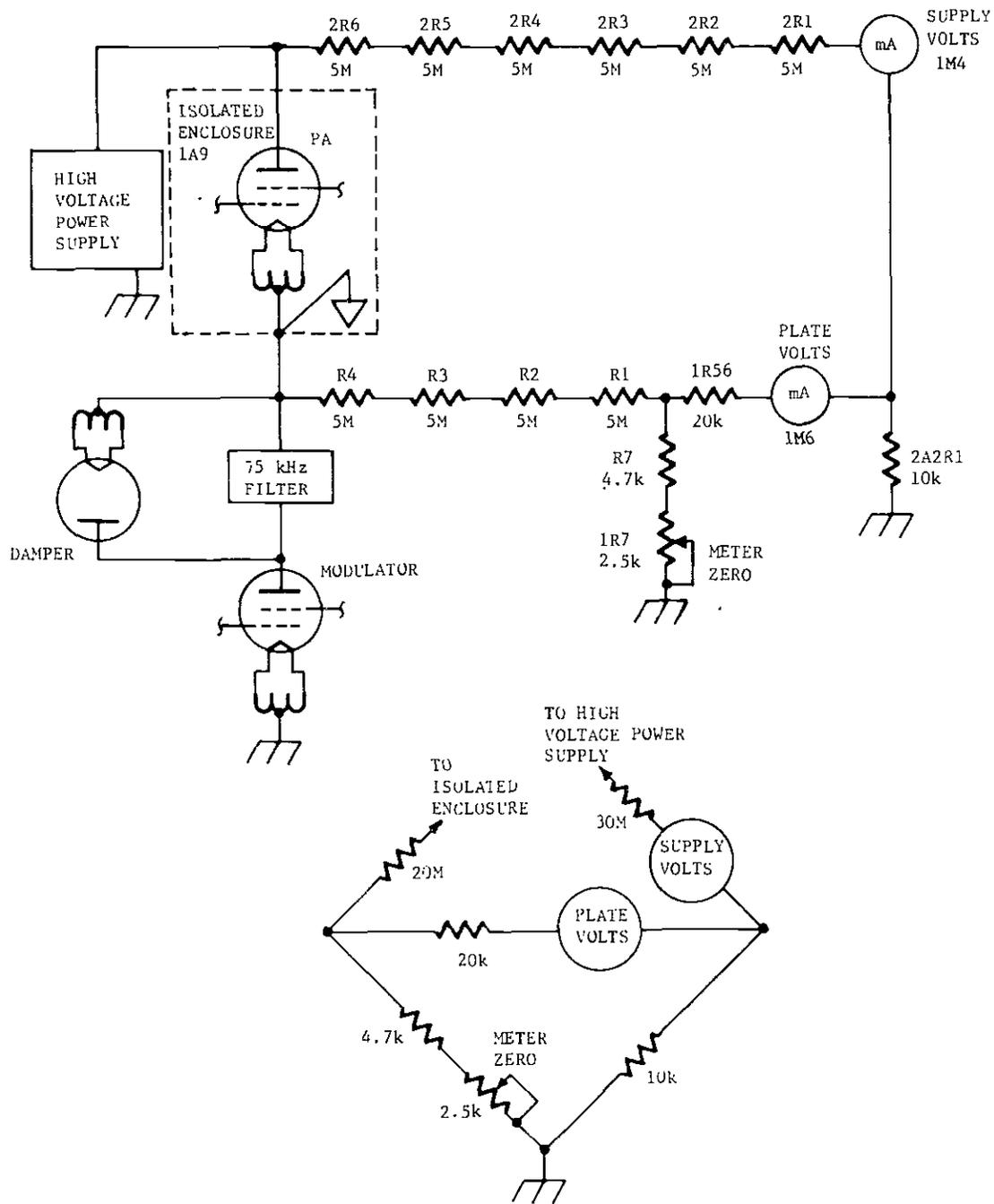
Figure 4-11. High Voltage Metering
