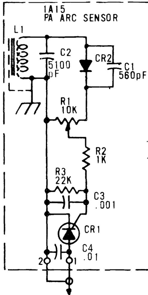
FIGURE 9-9. PA ARC DETECTOR
