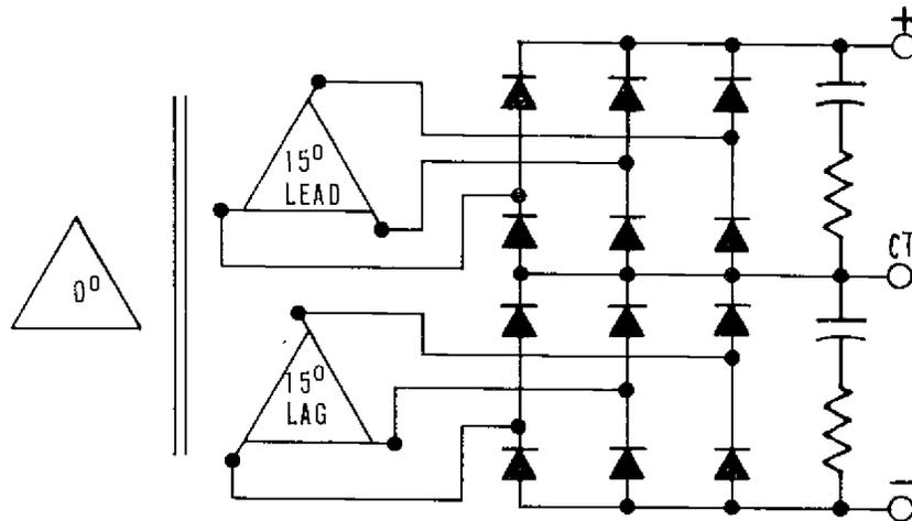
Figure 4-5. 12-Phase Circuit
