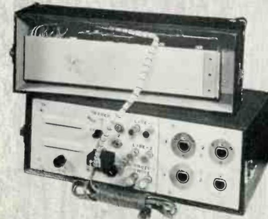
Battery pack plugs in back of amplifier which will always operate on A. C. until A. C. is interrupted—then changeover is automatic to batteries. Battery case section may be placed to the side or rear and need not be on top as illustrated above.
