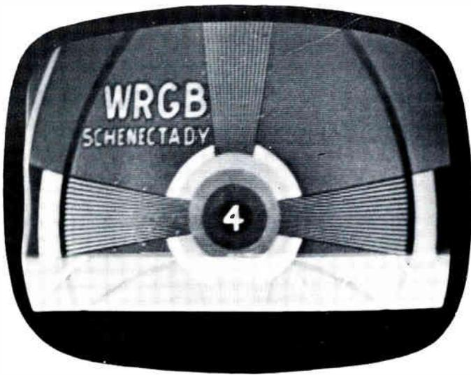
FIG. J-16. Foldover at bottom of picture due to leakage in capacitor C312.
