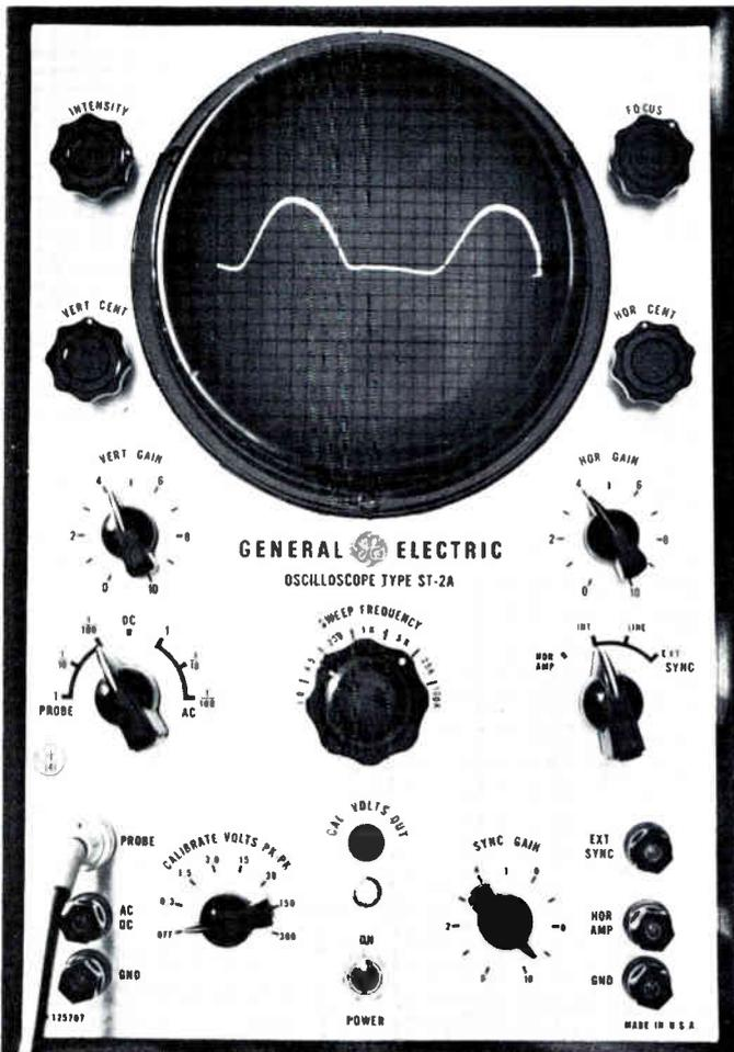
FIG. K-9. Waveform at point 2 in Figure K-1 with C365 open. The peak-to-peak voltage has dropped to about 100 volts.
