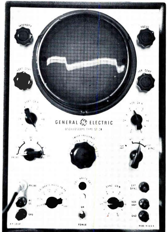
FIG. L-13. Normal waveform across capacitor C379A in Figure L-12. The peak-to-peak voltage is about 0.3 volts.
