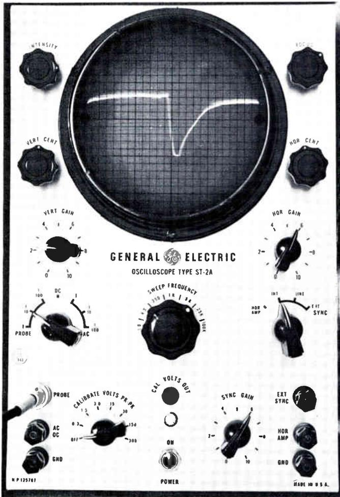
FIG. I-12. Waveform at point 1 with R357 open. The peak-to-peak voltage is about 30 volts.
