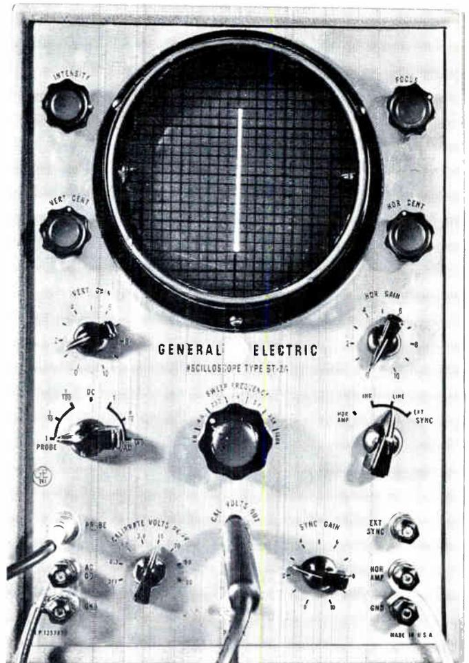
FIG. A-7. The General Electric Type ST-2A oscilloscope set up to indicate a peak to peak voltage of 15 volts or 1.0 volt per small square.
