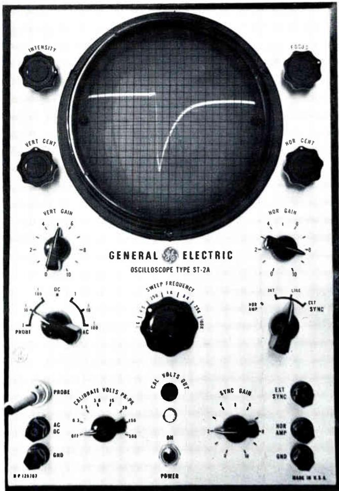
FIG. E-7. Normal waveform at point B in Figure E-1.
