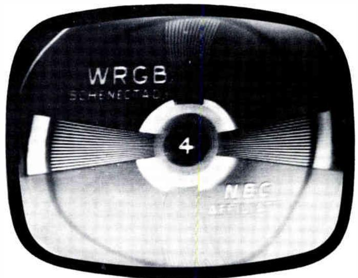
FIG. L-3. Test pattern somewhat more distorted due to heater-cathode leakage in one of the video i-f amplifiers. The weave in the picture is due to some of the hum getting into the horizontal circuit.
