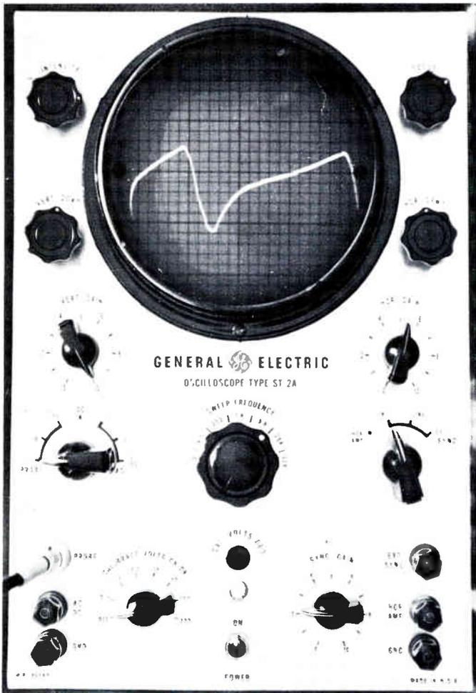
FIG. I-16. If capacitor C361 is open the waveform is changed but the amplitude is normal.
