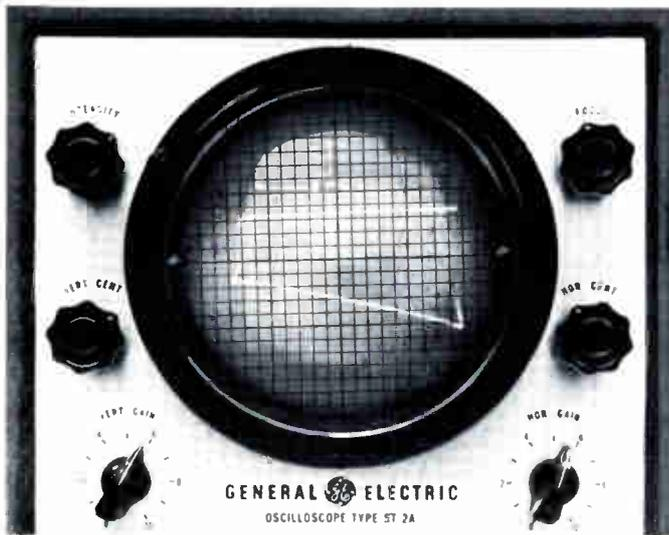
FIG. A-6. Normal alignment curve with the sweep width control in position #2.
