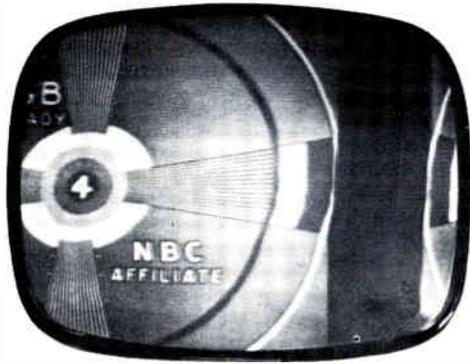
FIG. I-19. If capacitor C358 is open the picture weaves horizontally and will only stabilize with the blanking bar at the right side as shown or with a number of horizontal lines tearing the picture as appears in Figure I-20.
