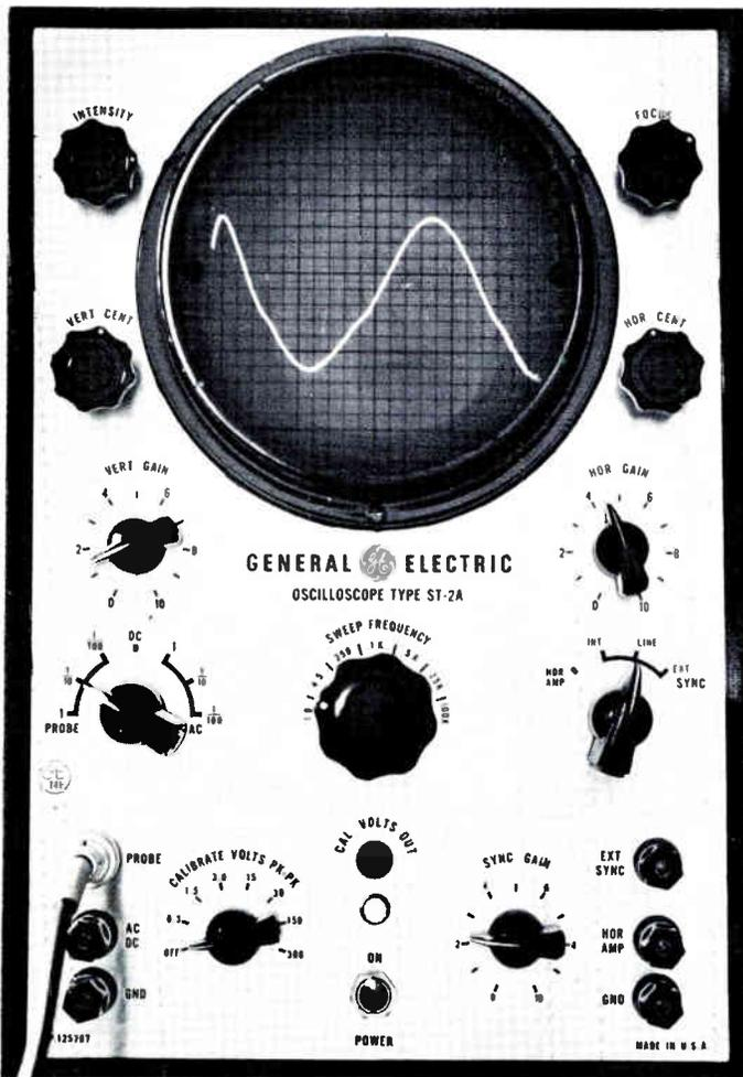
FIG. L-10. Waveform at point 4 in Figure L-1 if capacitor C453 is open. The peak-to-peak voltage has increased to about 42 volts.
