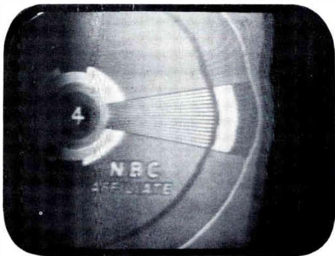
FIG. L-15. Test pattern with capacitor C379A in Figure L-12 open.
