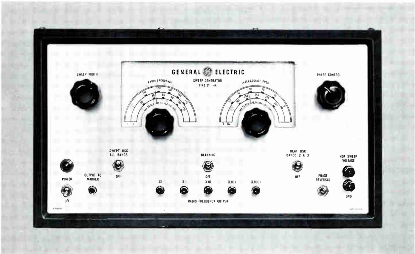
FIG. 9 The General Electric Model ST-4A sweep generator.
