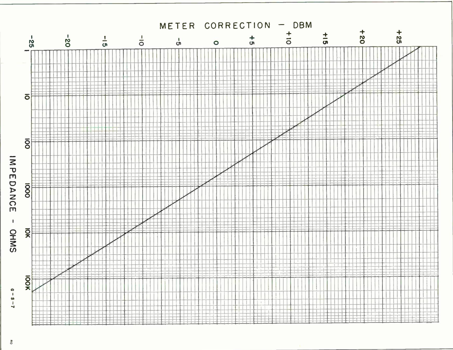
Figure 3-4. Impedance Correction Graph
