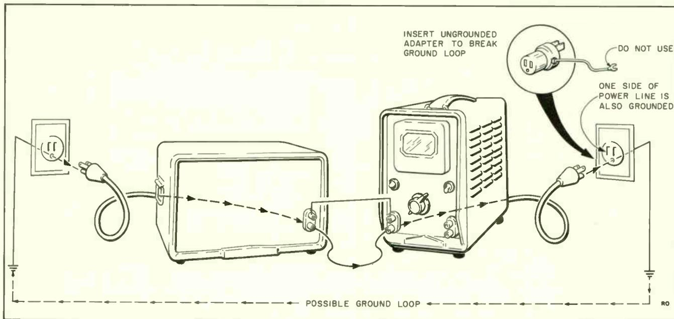
Figure 3-3. Test Setup for Avoiding Ground Loop
