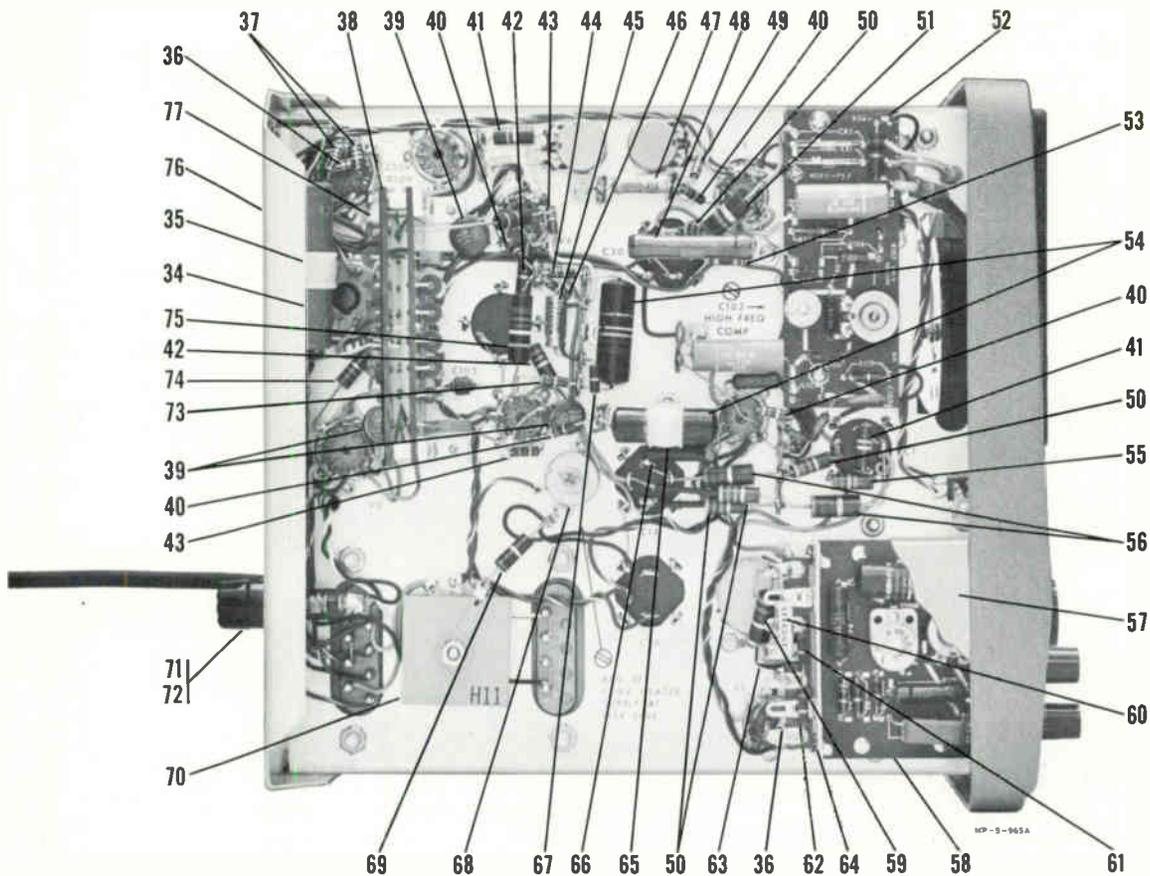
Figure 7-2. Main Chassis Assembly (Sheet 2 of 2)
