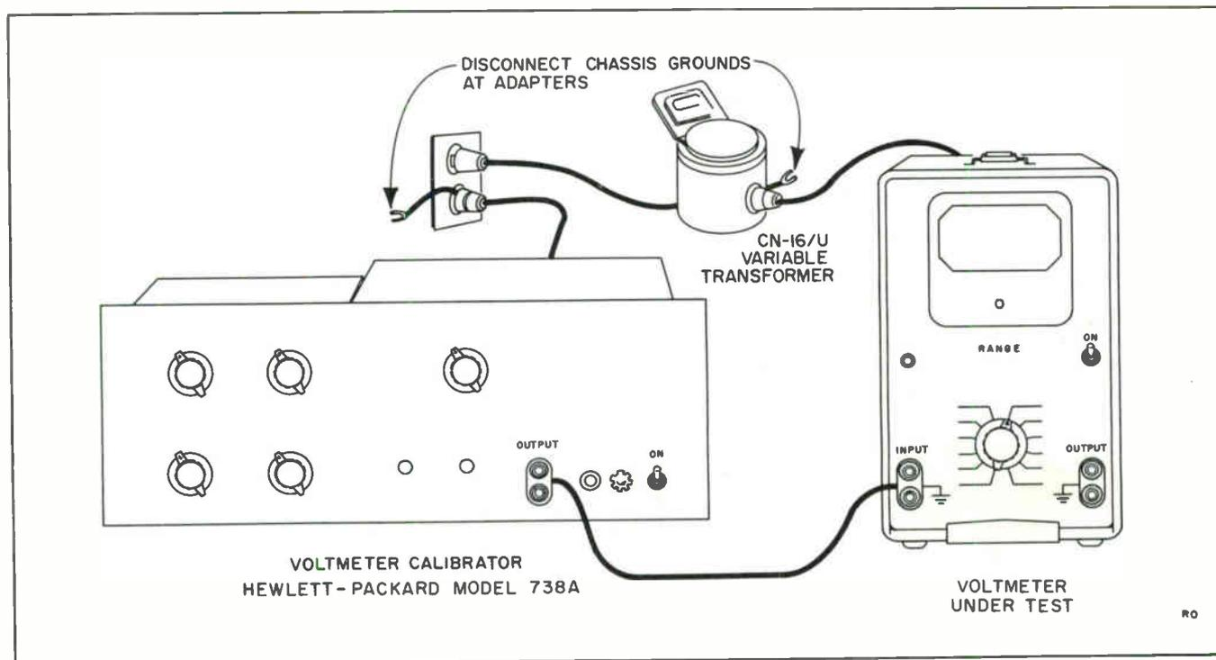
Figure 5-6. Test Setup for Calibration Check and Adjustments
