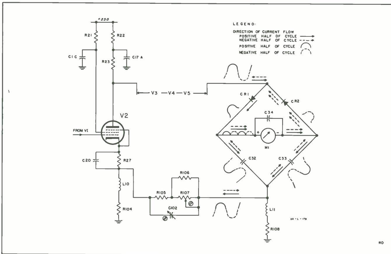
Figure 4-2. Simplified Schematic of Meter Bridge Circuit
