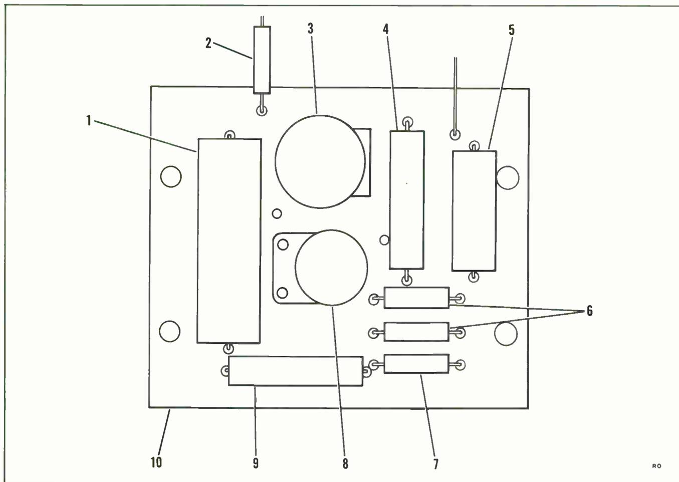
Figure 7-6. Printed Circuit Board Assembly, Part No. 400D-65C
