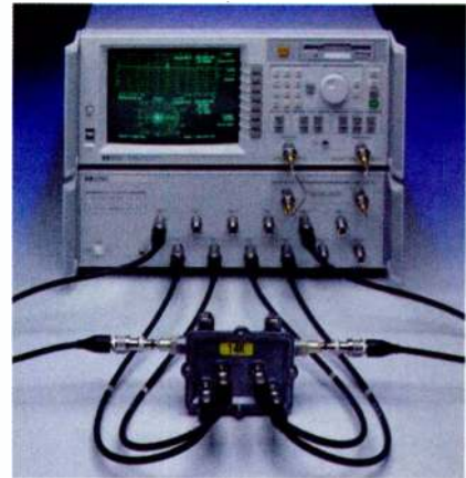
The HP 87075C multiport test set provides the fastest device measurement throughput available.
