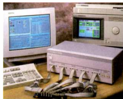
The HP E2474A 200-MHz state analyzer unit is designed to analyze fast host and cache buses.
