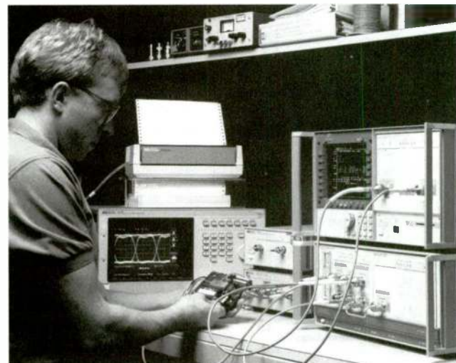
For lightwave applications, HP error performance analyzers cover rates to 12 Gb/s.
