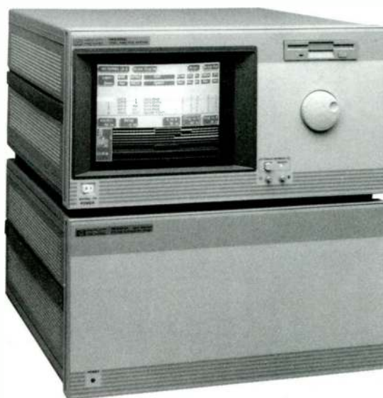
HP 16500C modular logic analyzer with color touchscreen, keyboard or mouse-driven user interface helps you quickly solve today's problems and provides room to grow in the future.
