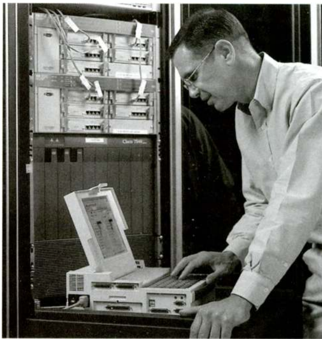
Portable protocol analyzer isolates operational problems on data communications networks.
