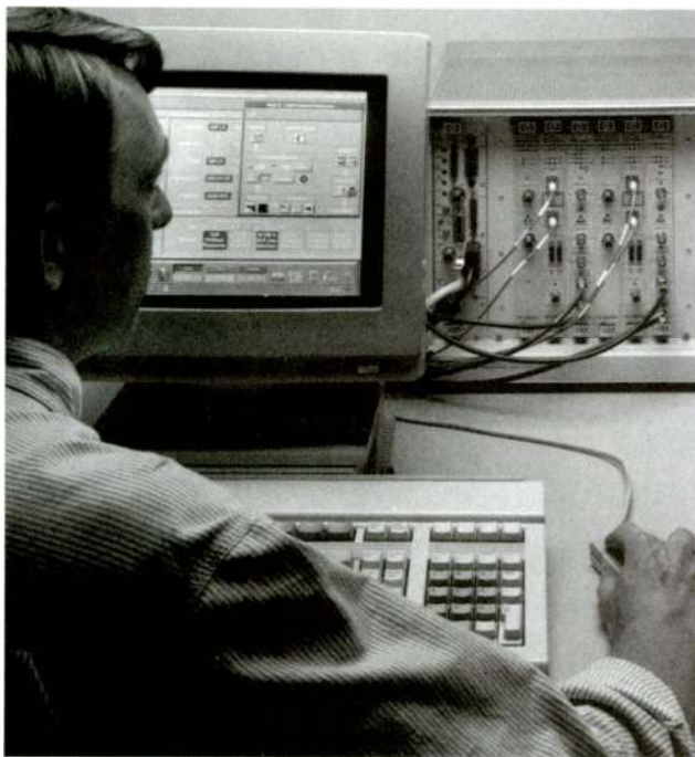
Broadband protocol testers handle ATM signaling and digital video testing.
