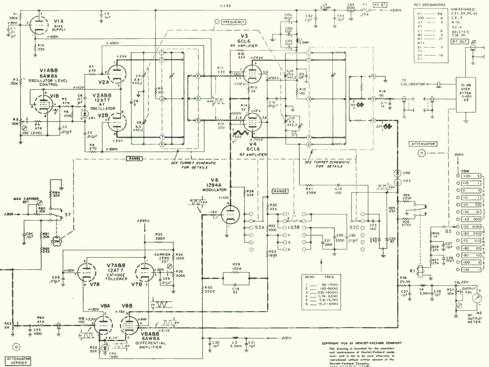
Figure 4-9. Signal Generator (Sheet 2 of 2)
