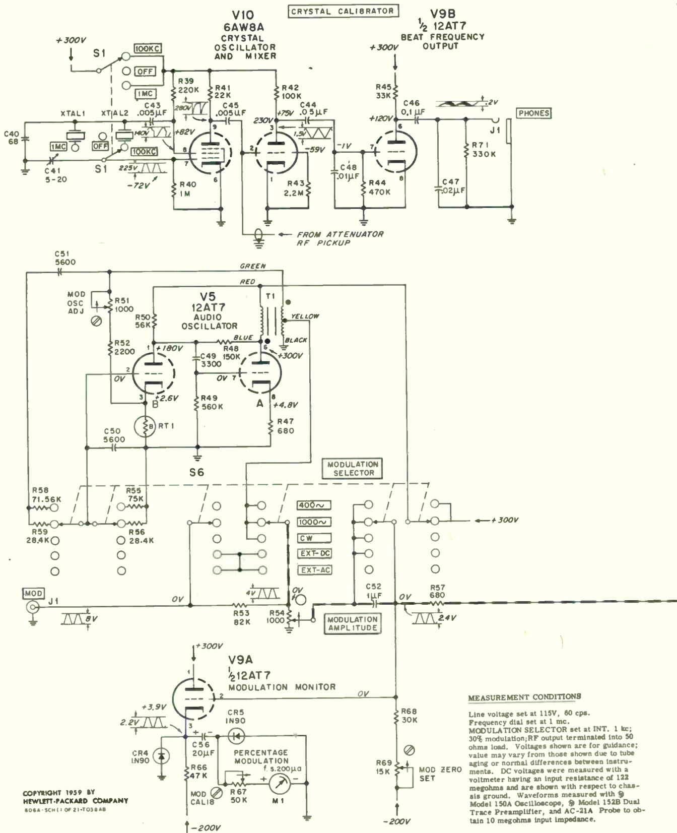
Figure 4-9. Signal Generator (Sheet 1 of 2)
