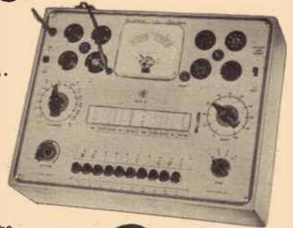
Test your tubes the modern way--dynamically--the simplest, yet fastest and surest method--your Heathkit has a switch for each tube element and measures that element--no chance for open or shorted elements slipping by, all the advantages of the mutual conductance type without the slow cumbersome time consuming setups.
