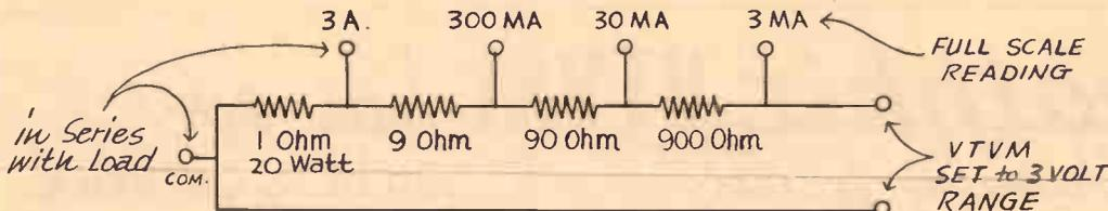
The resistors should be as accurate as possible. If used for AC measurements, the resistors should also be of a non-inductive type. In low voltage (filament or heater) circuits, the voltage drop across the resistors (3 volts at full scale reading) may be prohibitive, but in higher voltage applications this drop may usually be disregarded. For AC power measurements, the resistor network should be kept at the ground or low potential side.
