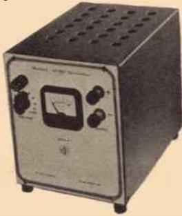
Even the smallest shop can afford the Heathkit Battery Eliminator Kit. A few auto radio repair jobs will pay for it. It's fast for service, the voltage can be lowered to find sticky vibrators or raised to ferret out intermittents. Provides variable DC voltage 5 to 7½ Volts at 10 Amperes continuous or 15 Amperes intermittent. Also serves as storage battery charger. Ideal for all auto radio testing and demonstrating.
