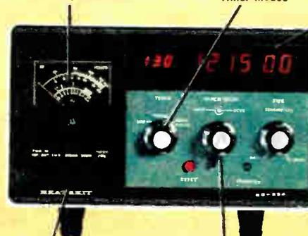
Adds real operating versatility to any station! The SB-634 features a 24-hour digital clock; ten-minute ID timer (with aural or visual alarm), RF wattmeter with 200 or 2000 watt full-scale ranges; an SWR bridge with sensitivity control; and phone-patch that can be used either manually or with VOX control. The wattmeter's impedance is a nominal 50 ohms and insertion loss is negligible. The phone-patch provides at least 30 dB of isolation between
