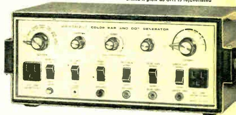
IG-5228 SPECIFICATIONS: Output signals: Video—Greater than  $\pm 1$  V peak-to-peak composite signal RF—Variable to 50,000  $\mu$ V output, channels 2 through 6. Sync.—Greater than 3.5 V peak-to-peak signal. Control Grids (3)—Individual red, blue, and green control grid signals for viewing chroma signal demodulator phase adjustments. Power supply: full wave zener diode regulated. Input—120/240 VAC, 60/50 Hz. Output—3.6 VDC, 300 mA, zener diode regulated. Dimensions: 5 1/2" H x 13 1/2" W x 8" D.
