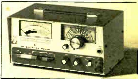
**IM-4180 SPECS:** Carrier Freq. Ranges: Fundamental, 25 to 50 MHz; Deviation Ranges: 0-2, 0-7.5, 0-20, & 0-75 kHz. Accuracy: ±3%. Full scale. Input Imped.: 50 Ω. Max. Input: 5 V. Scope Output: 13 mV/kHz peak.
