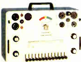
Test vacuum tubes on basis of total emission — for shorts, leakage, open elements and filament continuity.
