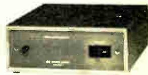
Designed to provide the 13.8 VDC required by the VF-7401, the VFA-7401-1 AC Power Supply may also be used with most other equipment requiring +13.8 VDC at a maximum of 3A continuous, 4A intermittent. Easy-to-build kit can be wired for either 120 or 240 VAC, 50/60 Hz. Output regulation within 1.5%. 3 $\frac{1}{16}$ " H x 7 $\frac{1}{4}$ " W x 9 $\frac{3}{8}$ " D.
