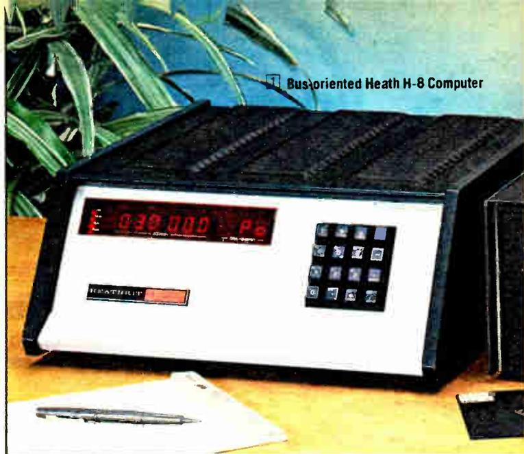
**Get added flexibility — at a budget-pleasing price:** The Heath H-8 Computer requires 16K bytes of Random Access Memory (RAM — see opposite page) and operating system software (Heath Disk Operating System/HDOS, the Heath/Zenith CP/M Operating System, the UCSD P-System with Pascal, H-8-18 Cassette Software or similar operating system — see p. 83 and check minimum memory requirements of each operating system) for normal operation.
