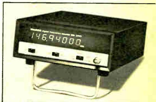
**IM-2410 SPECS:** Max. Sensitivity: 25 mV, RMS. Input Impedance: 1 MΩ shunted by less than 24 pF. Input Protection: 150 VAC, up to 100 kHz—derating to 5 VAC from 160 MHz to 225 MHz. Time Base Frequency: 3.58 MHz. Temperature Stability: ±10 ppm, from 0° to 40°C. Power Req: 120/240 VAC, 50/60 Hz. Dimensions: 3.38" H x 7.25" W x 9.5" D (8.59 x 18.42 x 24.13 cm).
