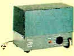
Provides the operating voltages for the HW-101 and other Amateur equipment. High voltage output is 700 VDC @ 250 mA; 300 VDC @ 150 mA and 250 VDC @ 100 mA low voltage taps. Provides fixed bias and 12.6 filament voltage. Excellent bias supply filtering and very low ripple. Overload protected. 120/240 VAC, 60/50 Hz, 350 watts max. 6 $\frac{3}{16}$ " H x 4 $\frac{3}{16}$ " W x 9" D.
