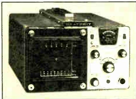
Following the tune-up specifications for any auto and using the Analyzer Operation Handbook, you can detect shorted spark plugs, bad points, defective wiring, worn distributor parts, incorrect dwell angle, cam wobble, plus coil or condenser defects and transistorized or capacitive discharge problems.
