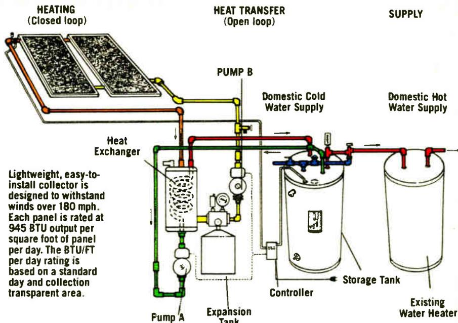
Lightweight, easy-to-install collector is designed to withstand winds over 180 mph. Each panel is rated at 945 BTU output per square foot of panel per day. The BTU/FT per day rating is based on a standard day and collection transparent area.
