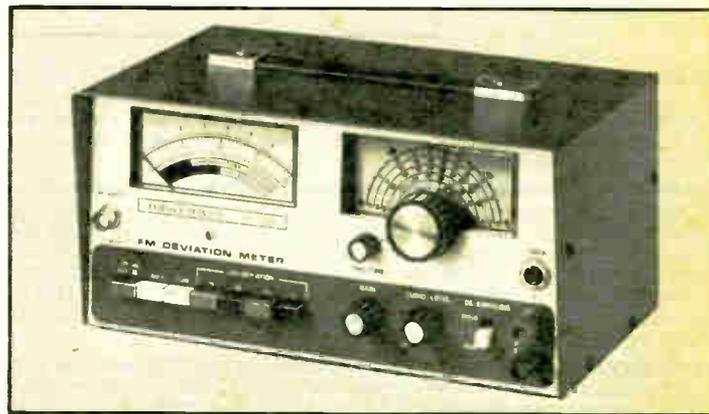
**IM-4180 SPECIFICATIONS:** Carrier Freq. Ranges: Fundamental, 25 to 50 MHz Deviation Ranges: 0-2, 0-7.5, 0-20 & 0-75 kHz. Accuracy:  $\pm 3\%$ , full scale. Input Imped.: 50 $\Omega$  Max. Input: 5 V Scope Output: 13 mV kHz peak.
