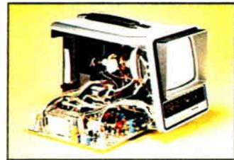
Pre-aligned modular circuit boards reduce assembly time and effort
