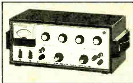
**A time-saving, low-cost addition to any audio test bench:** The IG-5218 provides both sine and square wave signals for gain & frequency response measurements, Harmonic Distortion checks and other amplifier tests. The square wave output with a risetime of 50 nanoseconds is ideal for audio response testing or as a trigger for digital circuit testing.
