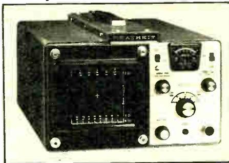
Following the tune-up specifications for any auto and using the Analyzer Operation Handbook, you can detect shorted spark plugs, bad points, defective wiring, worn distributor parts, incorrect dwell angle, cam wobble, plus coil or condenser defects and transistorized or capacitive discharge problems.
