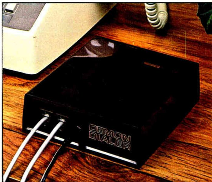
such as MCI, Sprint or ITT are offered, the Demon can dramatically improve your dialing speed and reliability by actually *detecting* dial and access tones instead of pausing. It's even portable—with built-in battery backup, directory memory is good for up to a year if unplugged from AC or four years with power.
