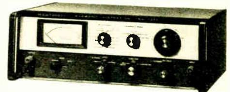
**IM-5258 SPECIFICATIONS:** Frequency Range: 5 Hz to 100 kHz in five ranges: 5-10 Hz, 10-100 Hz, 100-1000 Hz, 1-10 kHz, 10-100 kHz. **Distortion Measurement Ranges:** 0.3 to 100%, full scale, in six ranges with a 1-3-10 sequence. **Residual Distortion:** 0.03% or less. **Input Impedance:** 1 megohm, shunted by 70 pF maximum. **Required Input Level:** 316 mV RMS for distortion measurements
