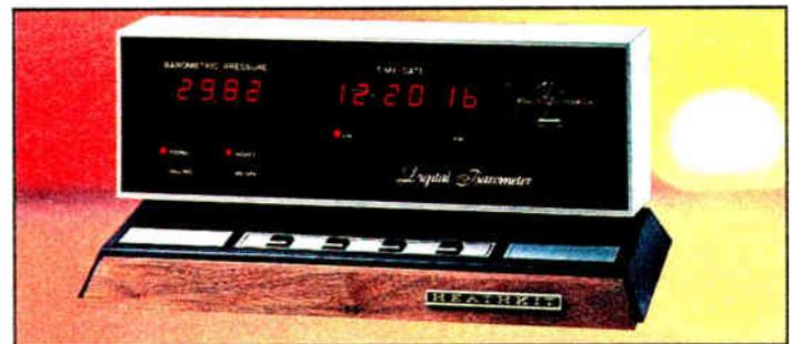
**ID-1990 SPECIFICATIONS:** Barometer Display: 4-digit readout. Separate indicators show whether the pressure is rising or falling, and whether the display is in inches of mercury, millibars or kiloPascals. Pressure Ranges: 28.00 to 32.00 inches Hg (mercury). 981 to 1050 millibars or 98.1 to 105 kiloPascals. Accuracy: 29.00 to 31.00 Hg ± 0.03 in. Hg at 15-35° C. Power: 120/240 VAC.
