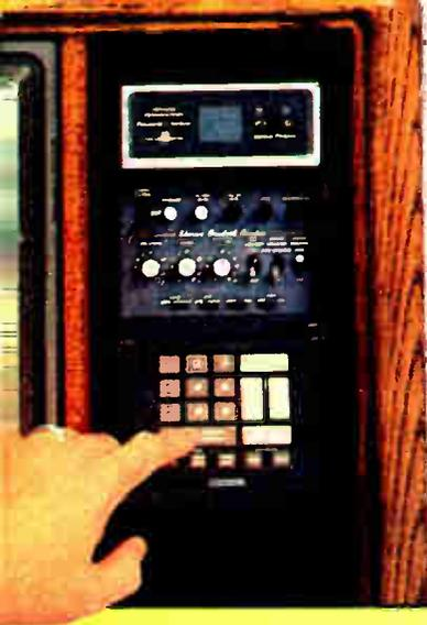
The GR-2502's hide-away control panel reduces tampering with TV adjustment. Quartz-controlled electronic tuning gets rid of the need for fine tuning and eliminates the normal wear-and-readjustment common with mechanical tuners. Select any channel being telecast in your area. A built-in computer selector instantly seeks out and locks on to the exact frequency. Have sharp, color-fast television at your fingertips or from a remote location! The panel closes for those fine adjustments.
