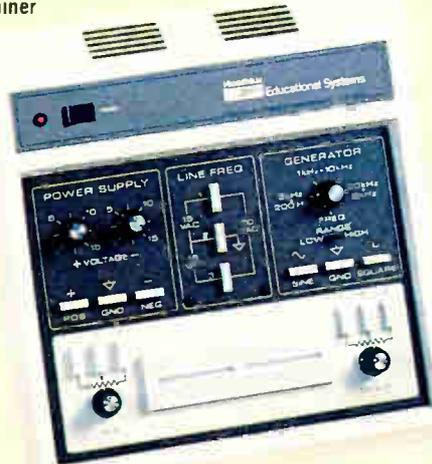
Solderless bread-board sockets for circuit building
