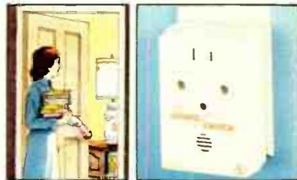
Provide extra safety in halls and on stairways. The Sound-Activated Switch turns on lights for you when you enter the area, and saves lots of money by turning them off after you've gone. Solves the problem of children-leaving lights on. Operates up to 300 watts of 120 VAC lights. Only two controls—sensitivity adjustment sets the sound-triggering level, and a timing adjustment sets turn-off delay.
