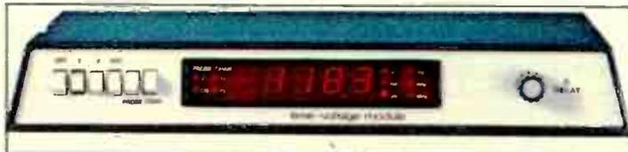
**Add-on Time-Voltage Module:** Used only with the IO-4360 Oscilloscope, the versatile IOA-4200 provides a 3 1/2 digit display of time, frequency or DC voltage measurements made with the scope's probe. Inputs are also provided on the IOA-4200 for making external voltage measurements up to  $\pm$  1000 volts DC. Bright LEDs are used to show all measurements with an automatic "-" being displayed for negative DC voltages. Low-profile cabinet mounts easily to scope.
