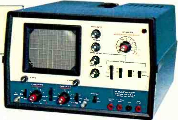
from 20 volts to 20 mV provides the scope with a wide variety of input ranges including variable gain control between settings. As with our more expensive models, a stable triggering circuit provides solid waveform displays. Trigger controls include selection of normal or automatic modes, switch controlled AC or DC coupling and input of external triggering signals. The time base is adjustable from 0.2 us/cm to 200 ms/cm plus variable control.
