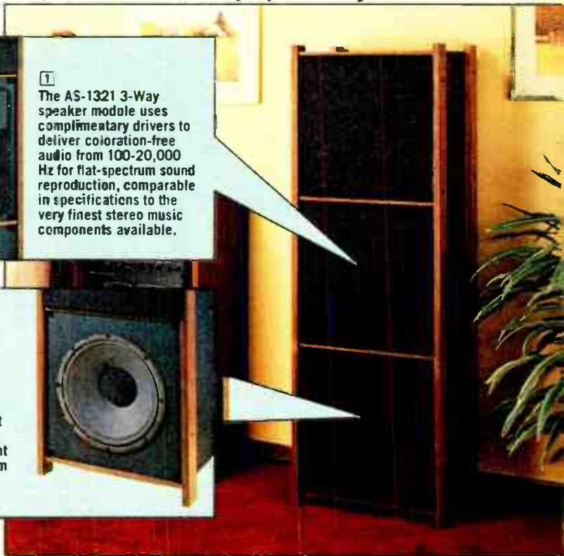
**AS-1320 SPECIFICATIONS:** Freq. Range (-10 dB anechoic): 15-750 Hz. Freq. Response ( $\pm 3$  dB): 22-500 Hz. Impedance: 8 $\Omega$ . Minimum Amplifier Power: 30 W. Maximum Power: 250 W. Driver: High compliance, 15" long-throw design. Cabinet Type: Nine-cubic-foot vented box, tuned to 22 Hz using computer-aided modeling techniques. Cabinet Dimensions: 64 $\frac{1}{2}$ " H x 21 $\frac{1}{2}$ " W x 17" D.
