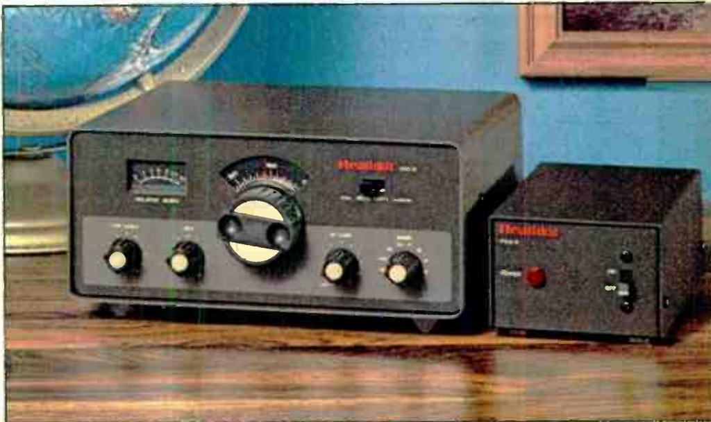
Detailed instructions take you through assembly and alignment, step by step. Only a VTVM or VOM, a frequency counter and dummy load are required to align the HW-9 Deluxe QRP CW Transmitter to specification performance.
